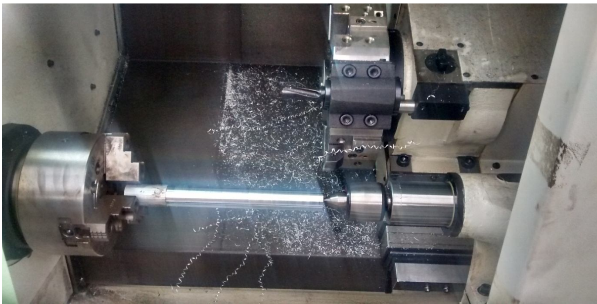
Fig 16 : Working of CNC turning in Metal Cutting Lab, DTU
