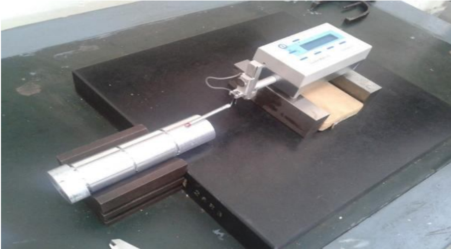
Fig 13 : Taylsurf instrument by Taylor Hobson Surtronic 3+ in Metrology Lab, DTU
