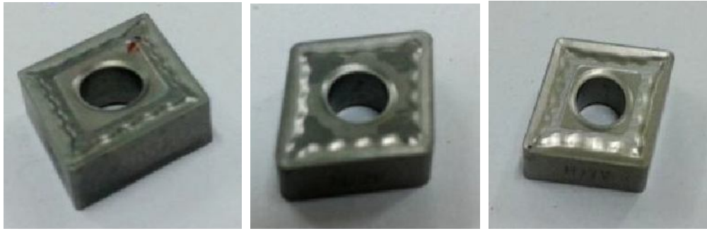
Fig 14:- Cutting tool-inserts (1.2mm, 0.8mm, 0.4mm)
