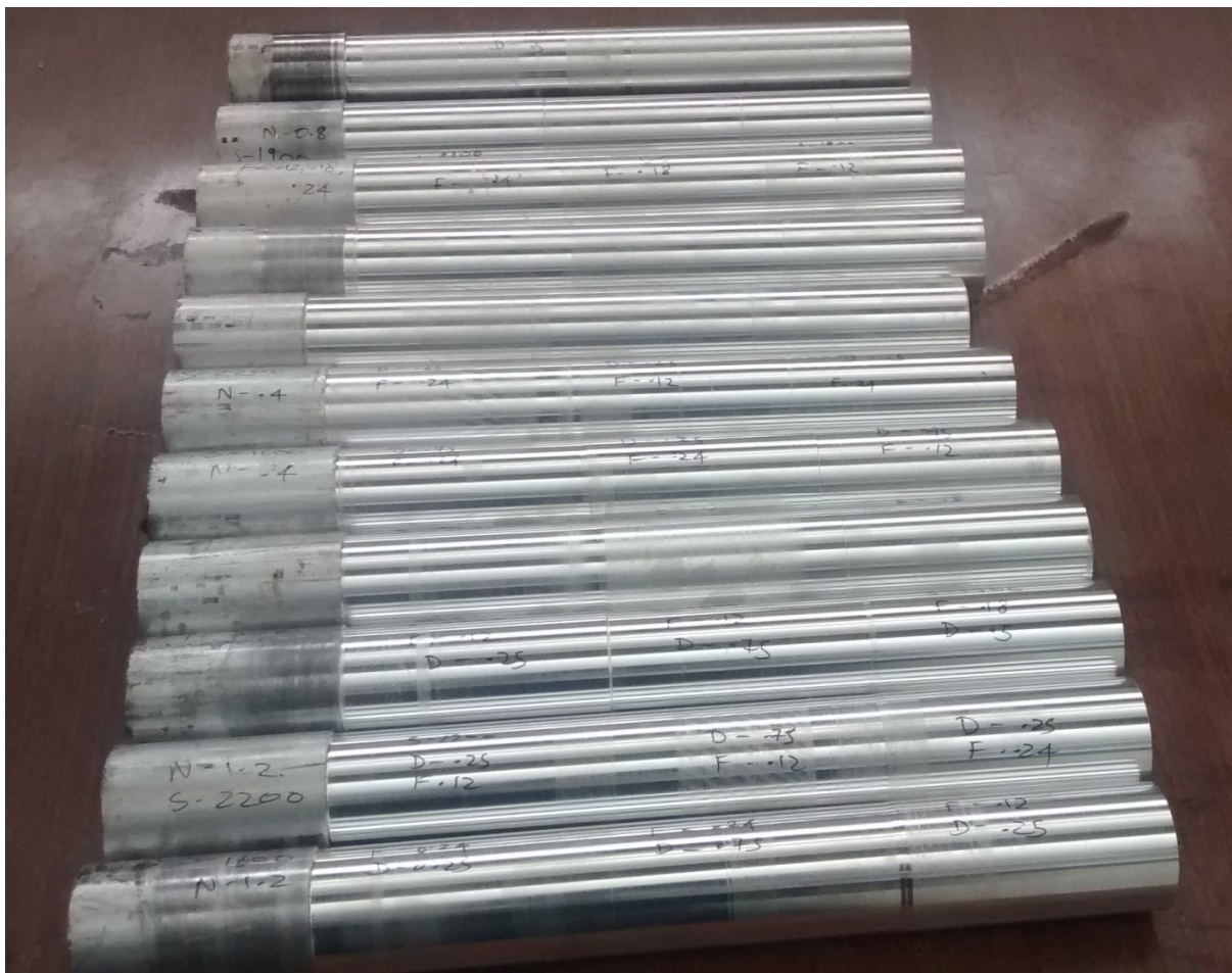
Fig 12 : Aluminium 6061 bars after turning at Metal Cutting Lab, DTU
