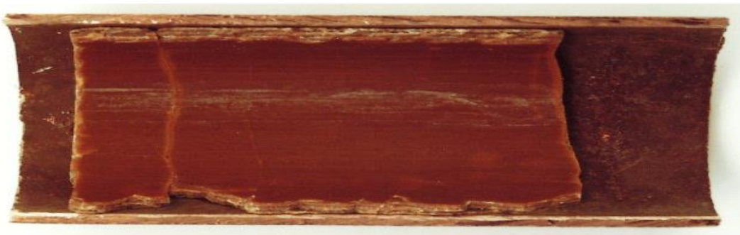
Figure 1.3: Condenser tube with calcium carbonate scaling. [14]
