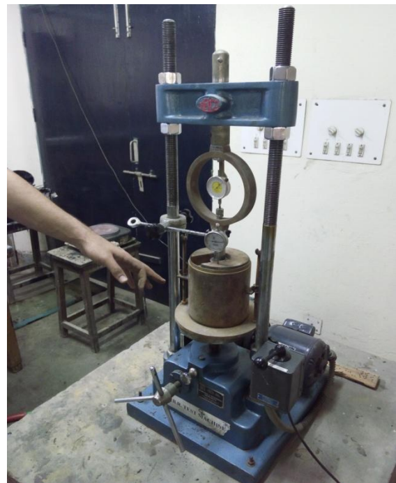
Fig.5.10 CBR test line diagram and set-up in laboratory
