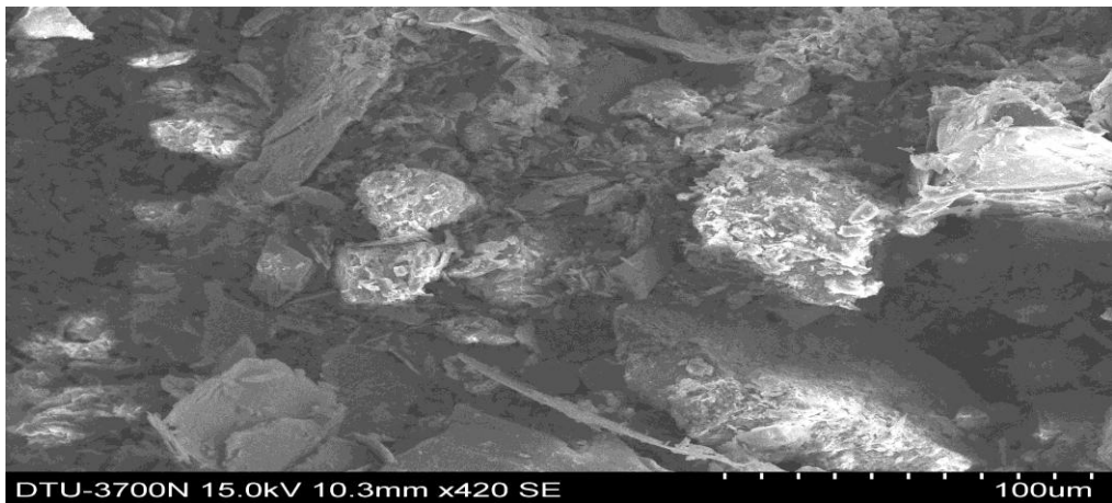
(b) SEM image of Sand at 100µm scale
