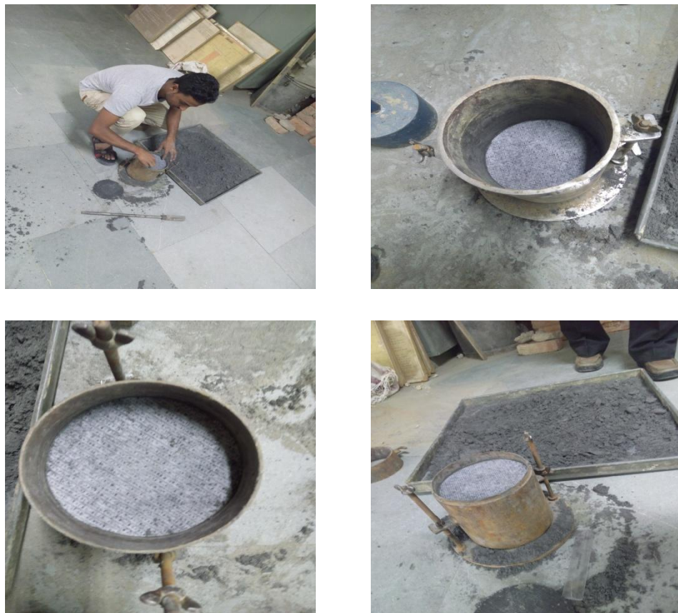
Fig.5.9 Preparation of pond ash beds and placement of reinforcement
