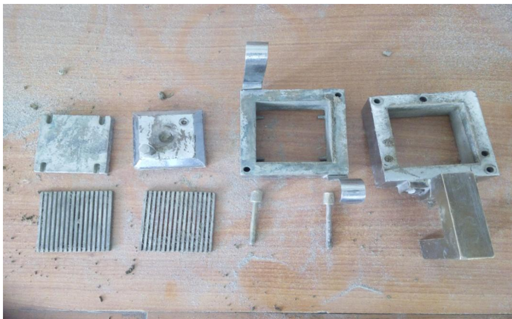
Fig.5.6 Components of direct shear test apparatus
