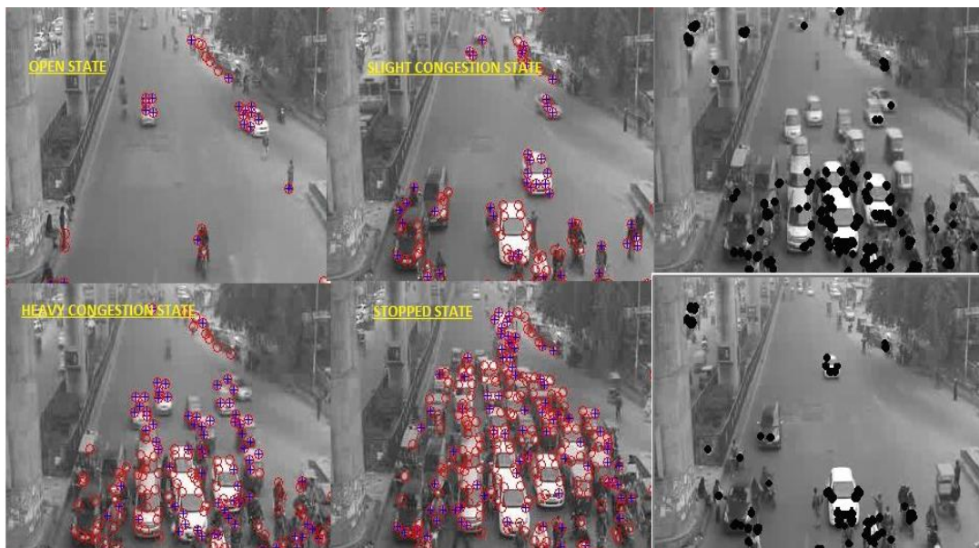
Fig. 10: Indication of traffic states obtained in different conditions using MATLAB and its implementation on hardware implementation using OpenCV(Indicated in last two images)
