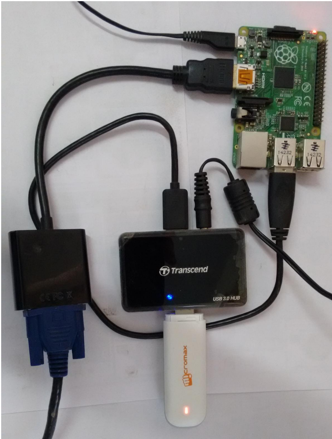
Fig. 29: Hardware for Raspberry Pi to 3G modem interfacing
