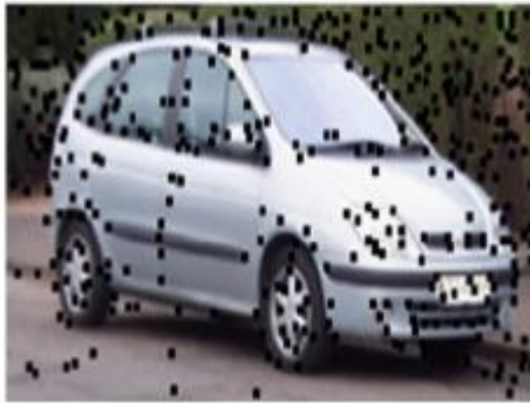
Fig.3.2.1. interest points extracted from highly textured parts and those from abrupt changes.
