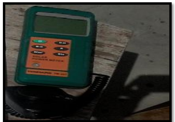
Figure 16: Solar Power Meter (Tenmars TM-207)
