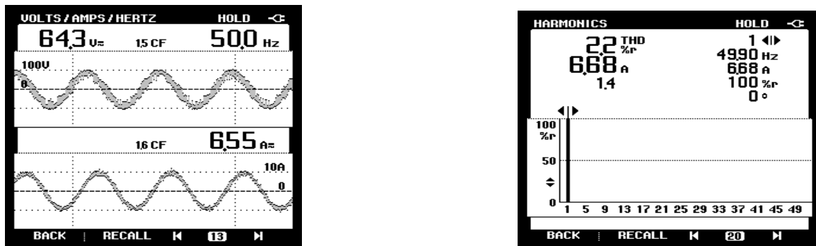
Fig 5.18 Source current and its THD after compensation using Anti-Hebbian algorithm based controller
