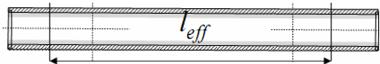
Fig 1.5: Definition of the effective length[6]
