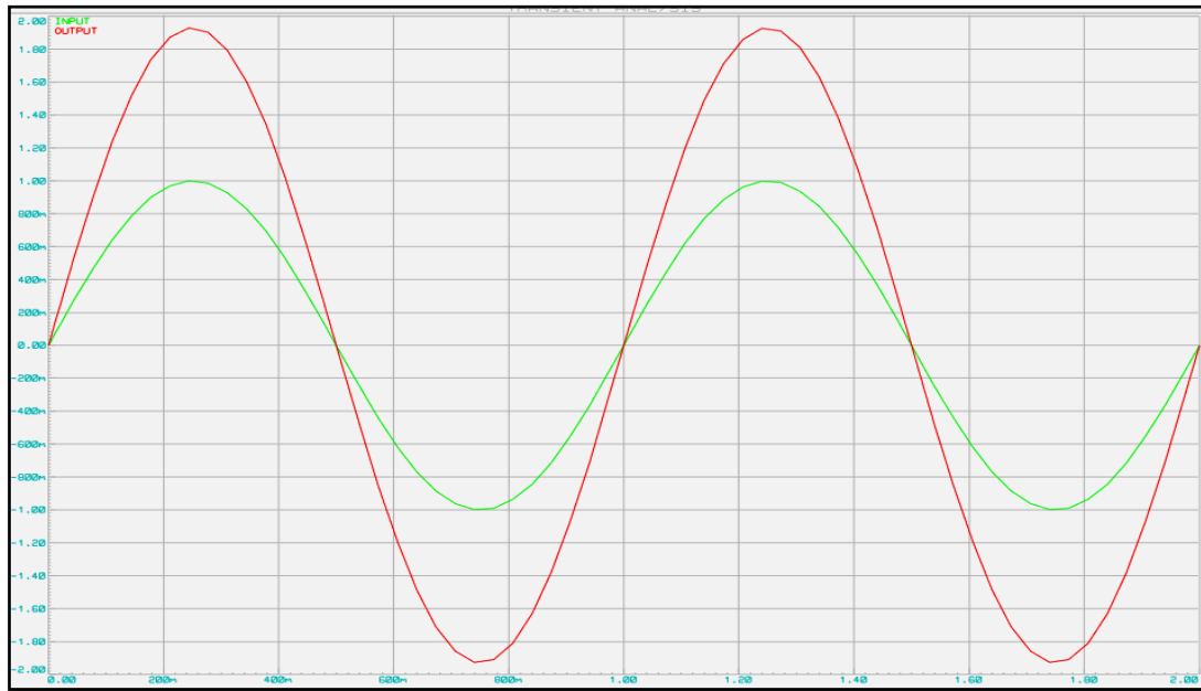
Figure 6.5 Transient response of P - Controller
