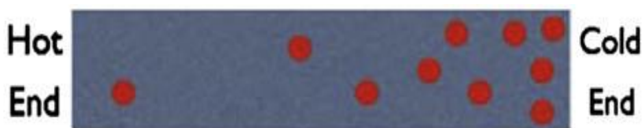
Figure 2.1: Charge transportation from the hot to cold end for negative Seebeck co-efficient materials [8].
