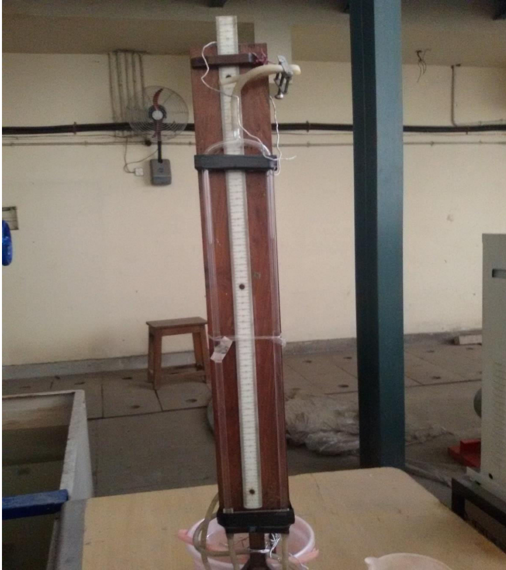
Fig. 3.2.1 (a) INVERTED U-TUBE MANOMETER WITH WOODEN STAND
