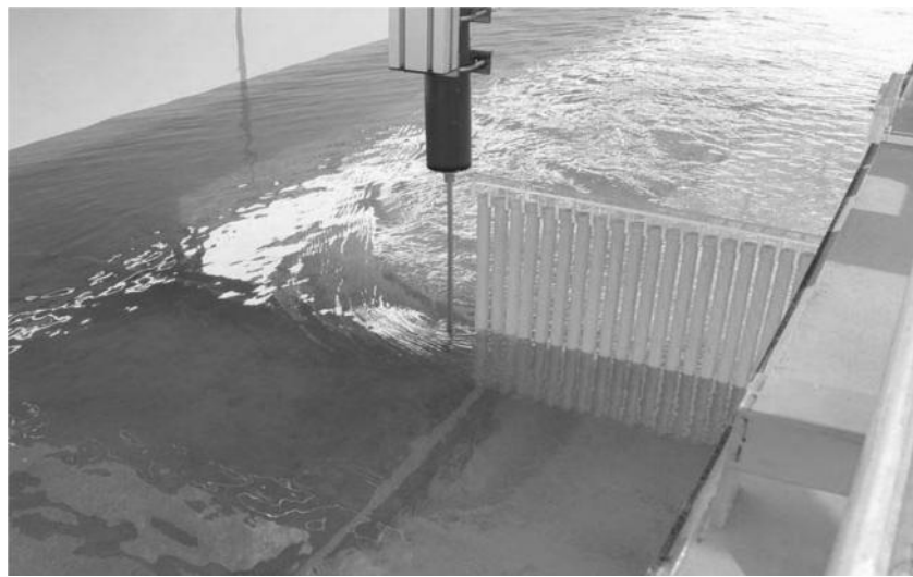
Fig.3.3 The Tip Velocity measurement by ADV
