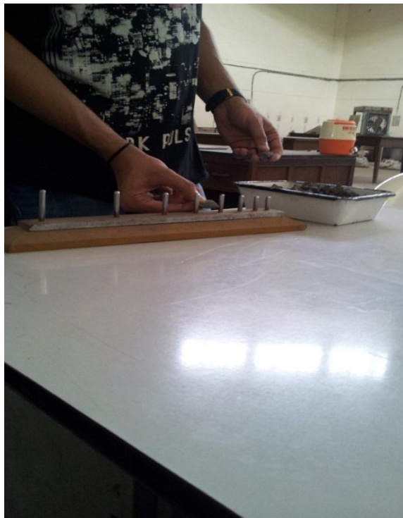
Figure 4.4: Length Guage for determining Elongation Index
