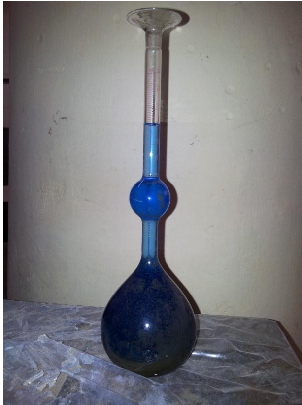
Figure 4.8: Le Chatelier's flask filled with kerosene for calculating specific gravity of cement.
