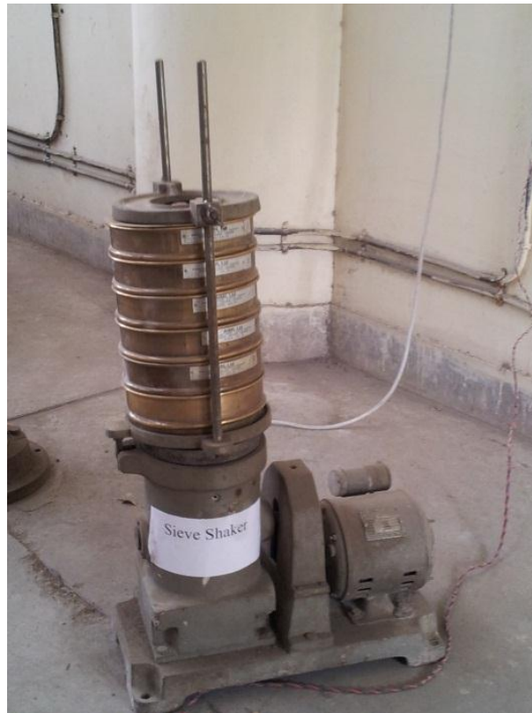
Figure 4.1: Using of Sieve Shaker for sieve analysis
