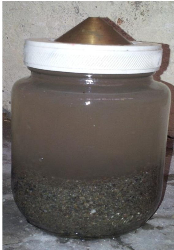
Figure 4.7: Using of Pycnometer for determining specific gravity.
