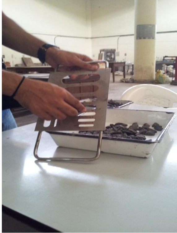
Figure 4.3: Metal Guage for calculating Flakiness Index
