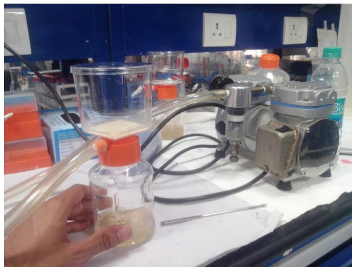
Fig. 10 Filtration of cell free extract with 0.22 \mu\text{m} filter with filtration assembly
