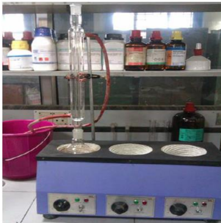
Figure:6 Assembly for preparation of porphyrin
