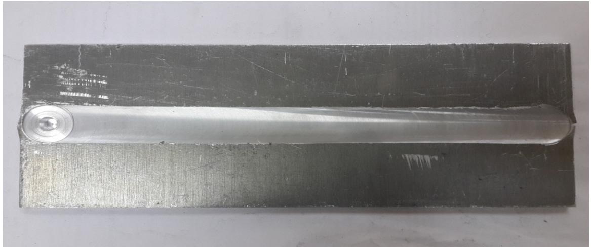
Figure 24-Friction stir welded AA6082 plate
