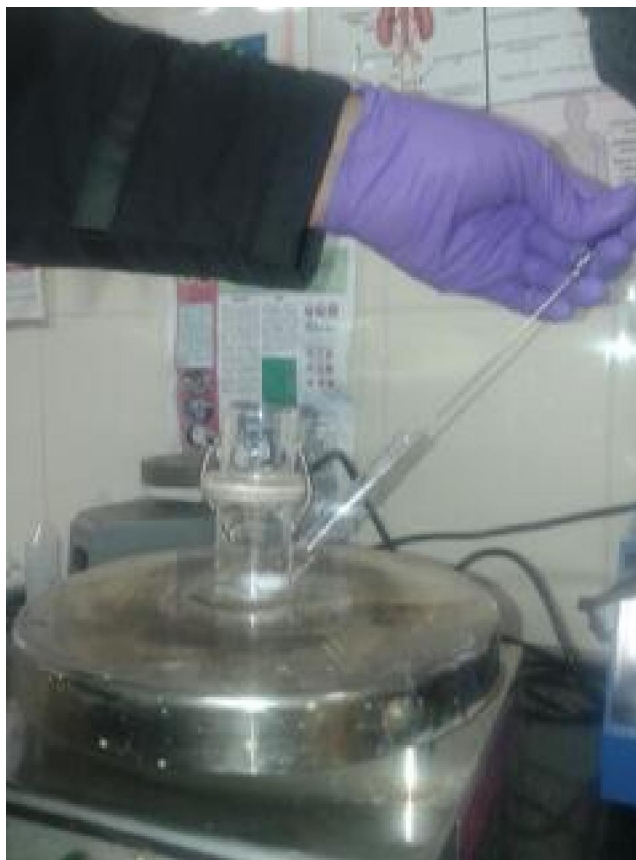
Figure 6. Extracting the aliquots from Franz Diffusion Cell
