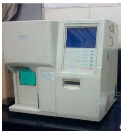
Fig 10: Sysmex XE-2100 automated hematology system for blood cells count
