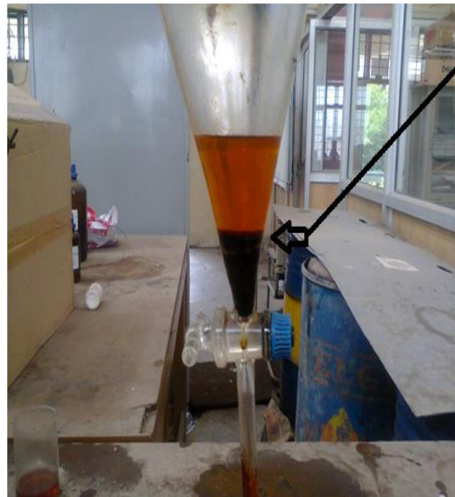
Fig.3(h) Second Stage Separation After Alkaline Transesterification
