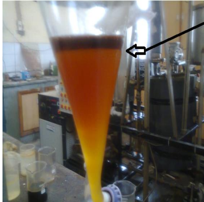
Fig.3(g) First Stage Separation After Acid Esterification
