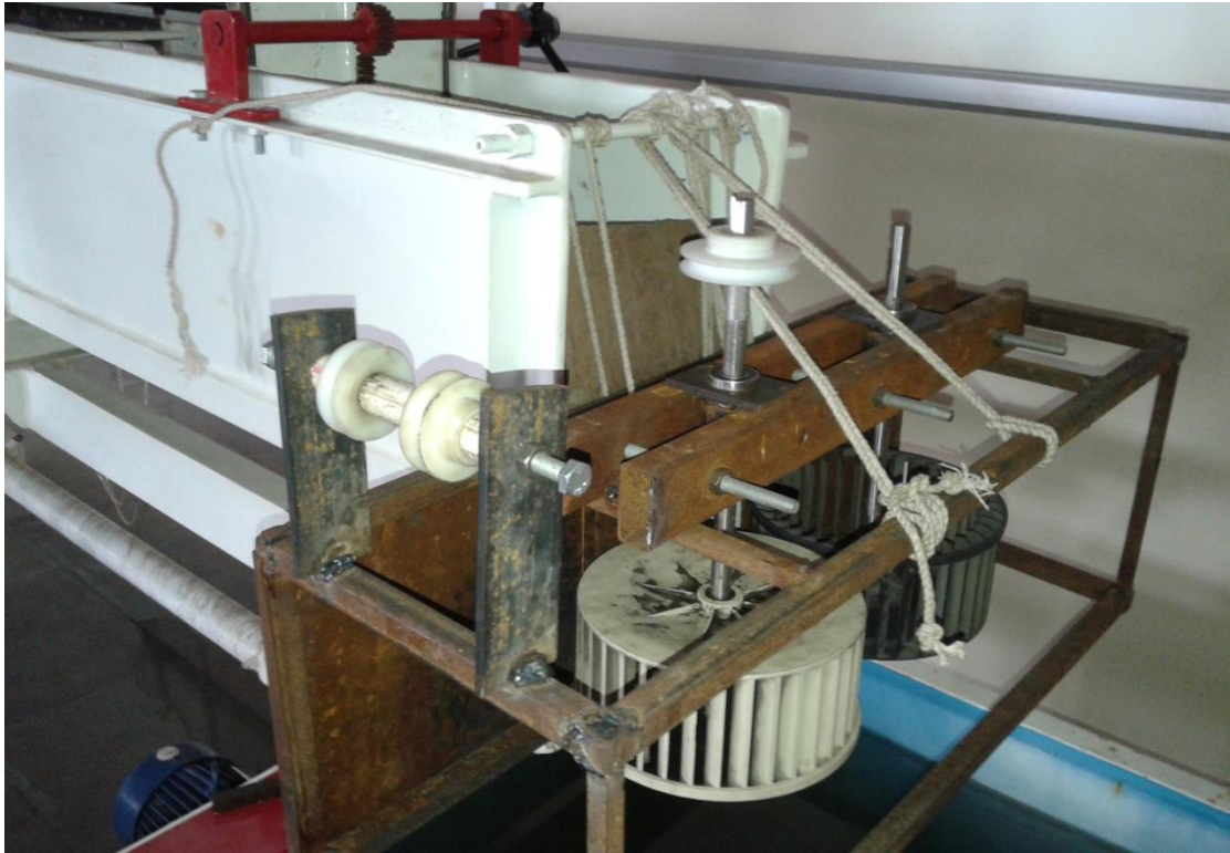
Fig. 5 Assembly of plume channel set-up with runner assembly
