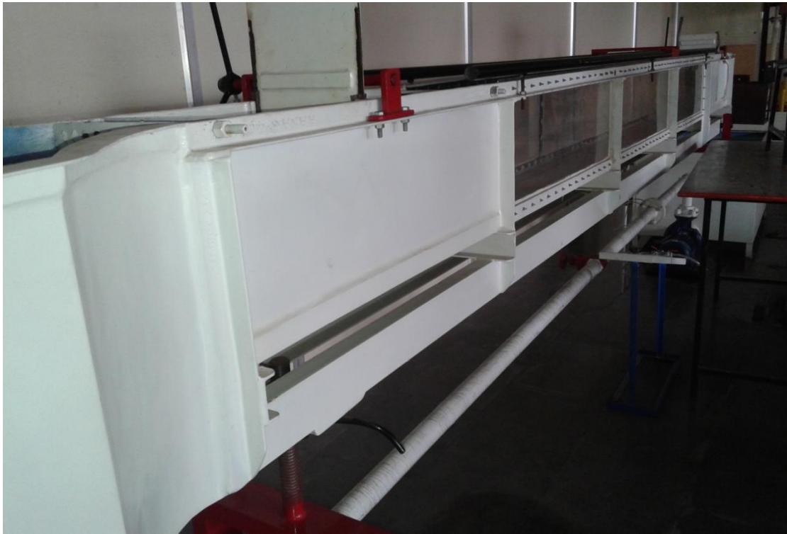
Fig. 4 Assembly of plume channel set-up
