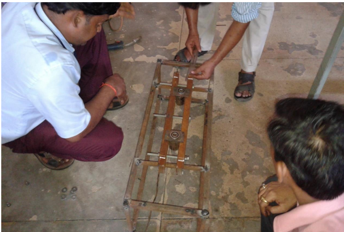
Fig. 6 Stand assembly for runner fixing
