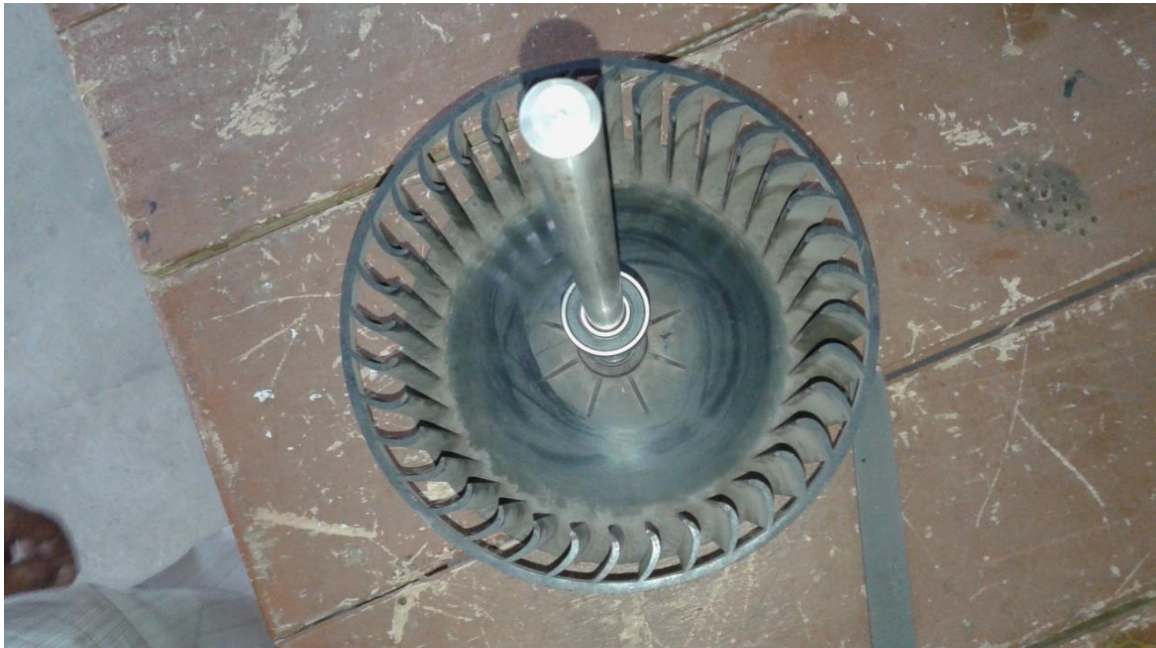
Fig. 2 Runner and shaft assembly top view
