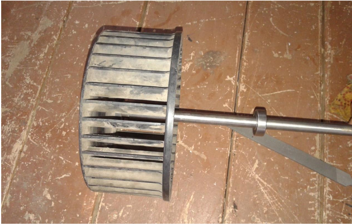
Fig: 1 Runner and shaft assembly side view
