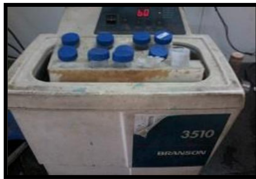
Figure 18: BRANSON Sonication device
