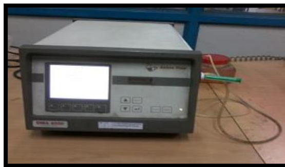
Figure 22: Density Meter (Anton Paar-DMA 4500)
