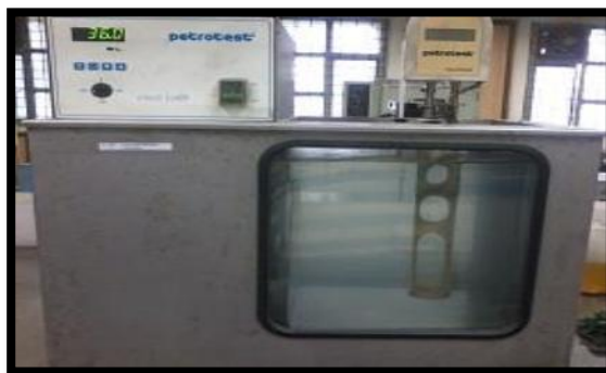
Figure 23: kinematic viscometer (Petrotest Viscobath)
