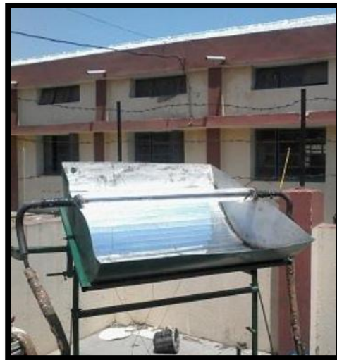
Figure 15: Side view of PTC system
