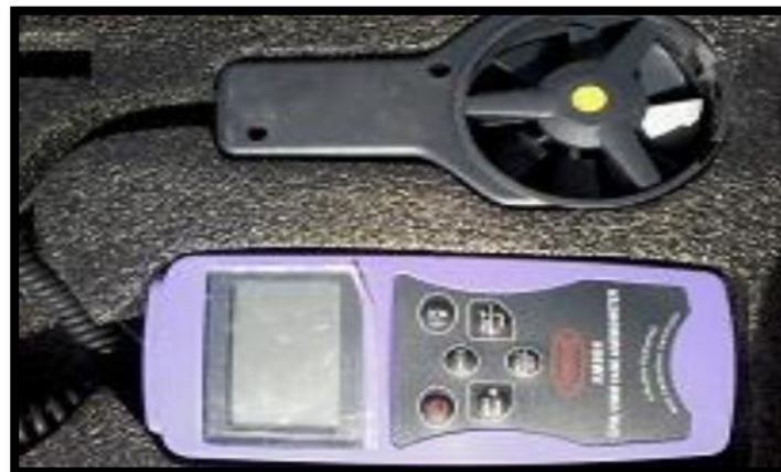
Figure 17: CFM/CMM Vane Anemometer (PRECISE AM804)
