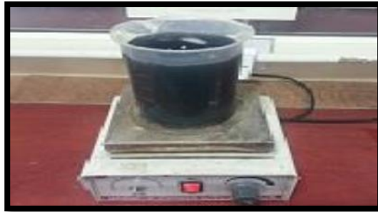
Figure 19: Magnetic stirrer with hot plate
