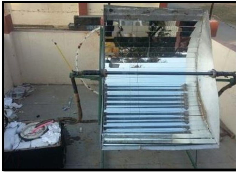
Figure 13: Front view of experimental set up of PTC system (Thapar University)
