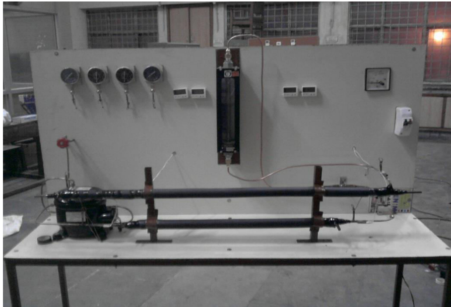
Fig.4.1 Vapour compression refrigeration system model
