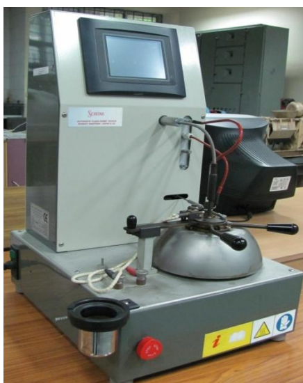
Plate 3.8 Pensky Marten Flash Point Apparatus
