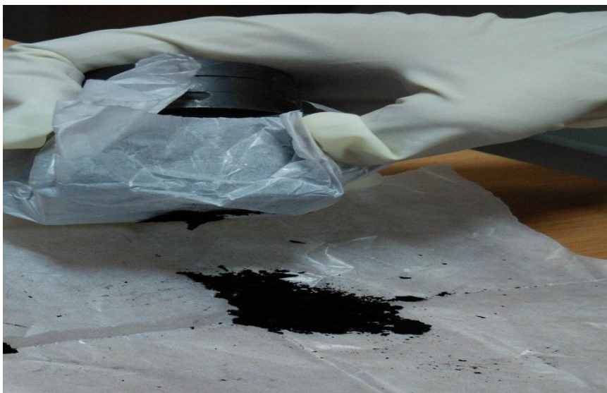
Figure 4.6. Removal of non magnetic elements from the as-obtained sample
