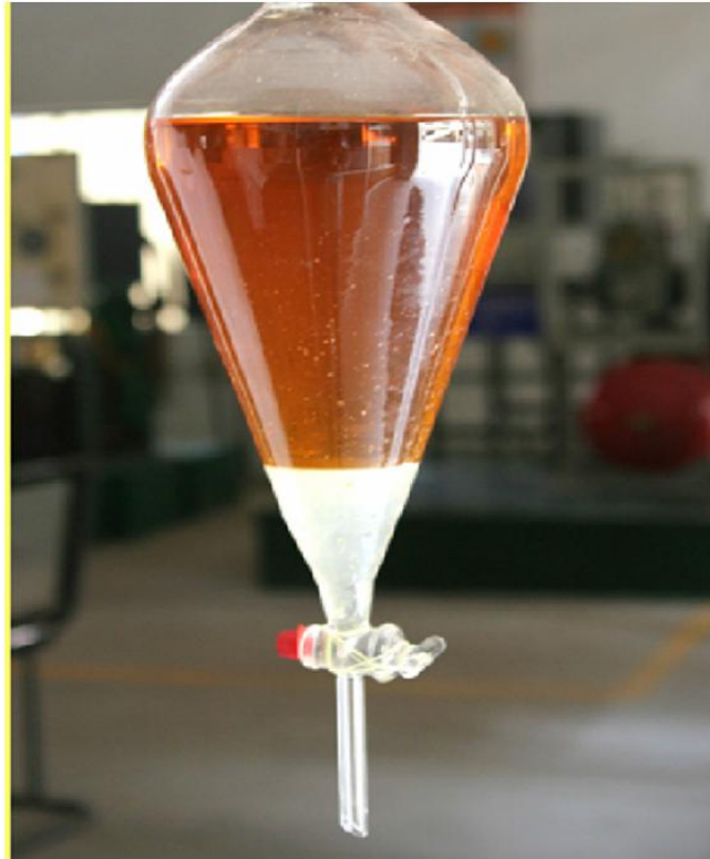
Fig.4. Pure bio-diesel at top layer & clear water at bottom layer.
