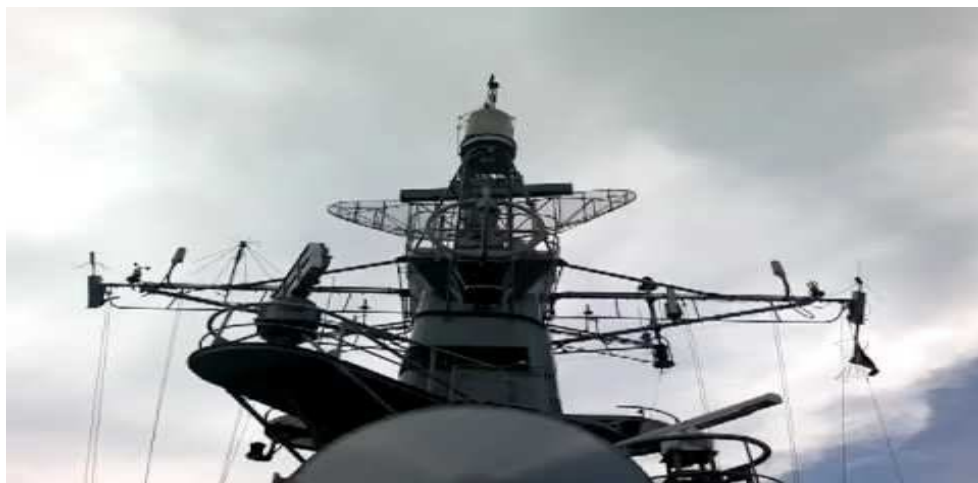
Figure 1.1 Ship's mast containing RADAR and communication antennas
