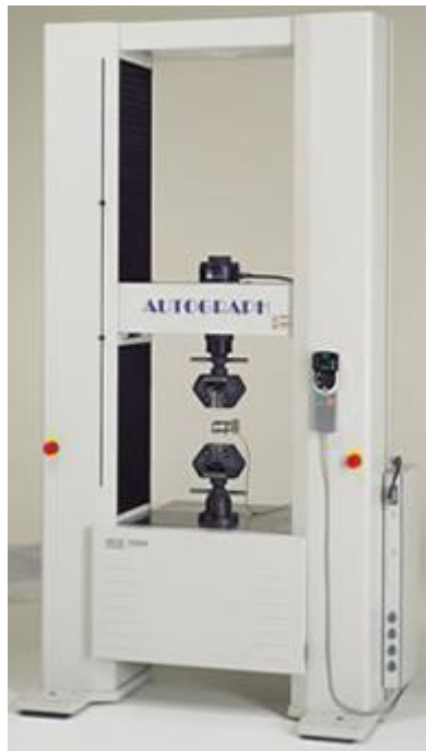
Figure 3.6: Universal Testing Machine
