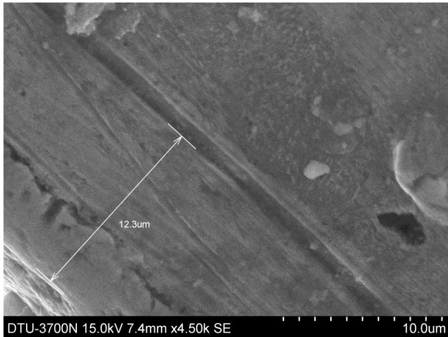
Figure 4.2: (b) Cross-sectional view of Ion-Plating at 10 \mu\text{m}
