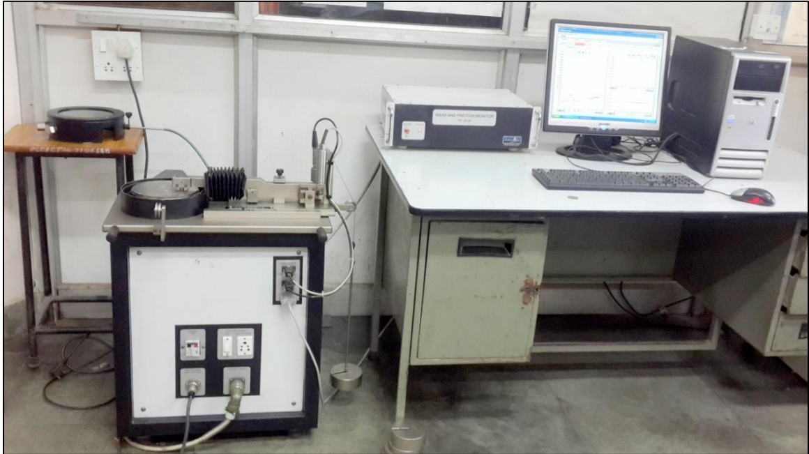
Figure 3.3: Wear and friction monitor machine for pin on disc test
