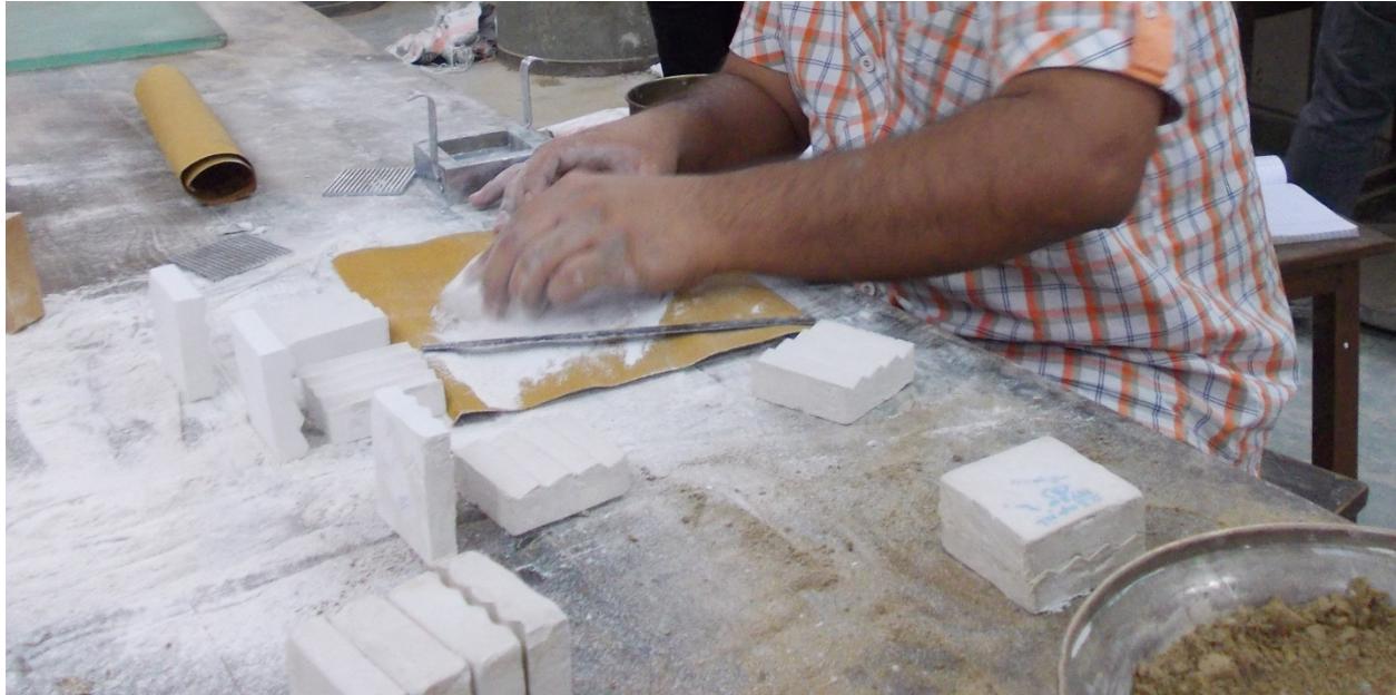
Fig 3.1: Shows the Sample of direct shear test made up of Plaster of Paris.
