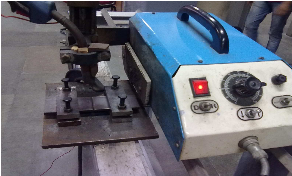
Fig4.4:- Motor Driven Trolley
