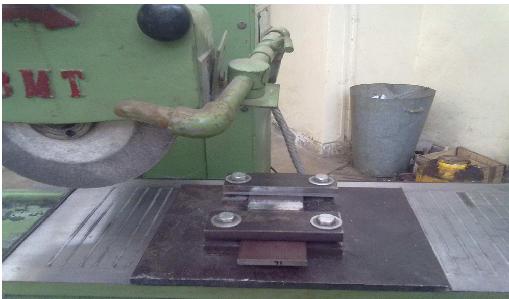
Fig 5.4:- Grinding in progress
