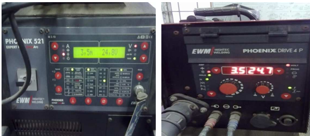
Fig 4.2:- Control panels of phoenix 521expert force arc MIG/MAG machine.
