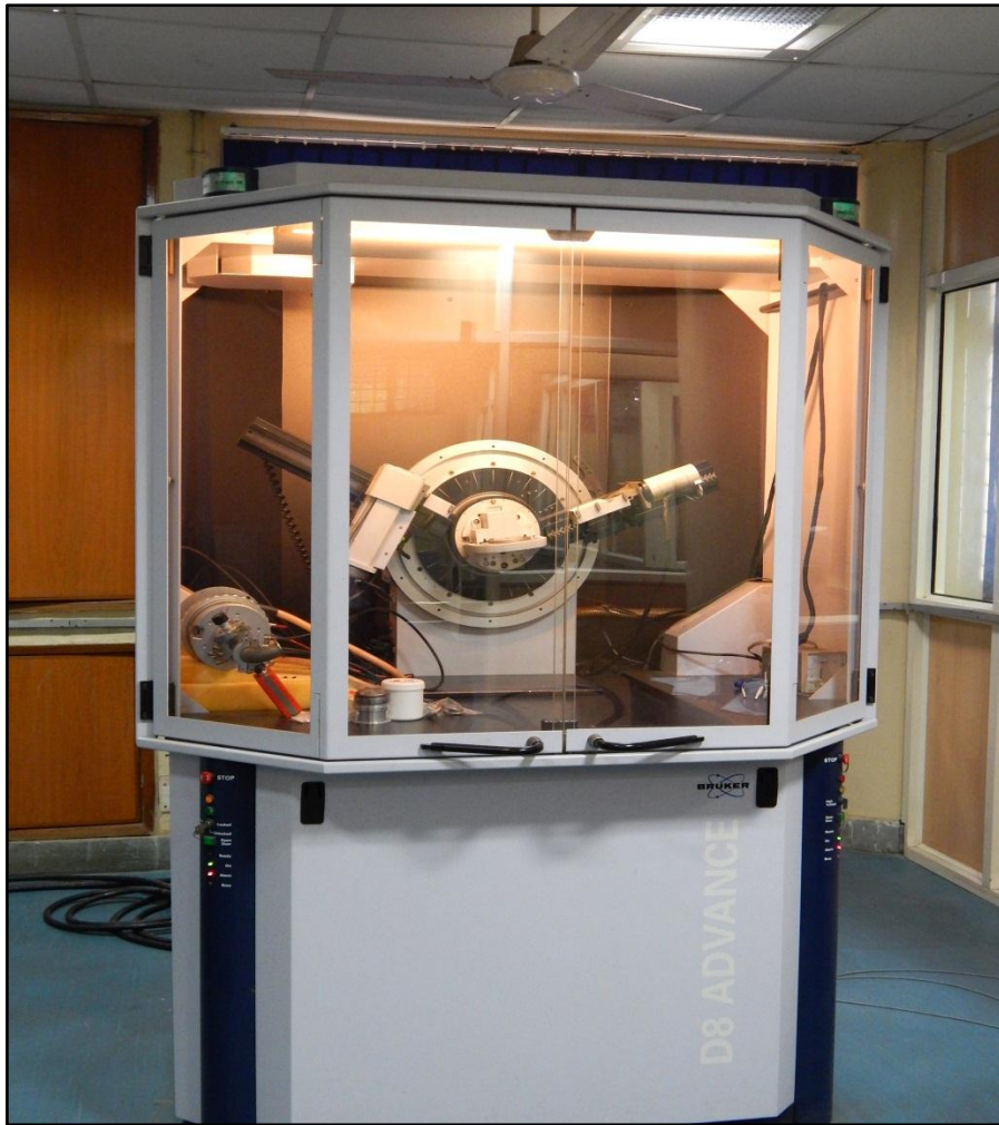
Fig 12 XRD Apparatus in our Nano Lab
