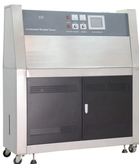
Figure 3.6 UV Weather Resistance Test Chamber
