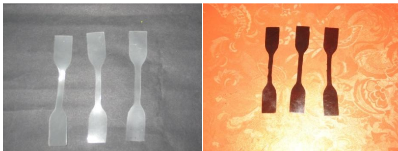
Figure 3.4 Dumbbell shaped specimens before and after radiation
