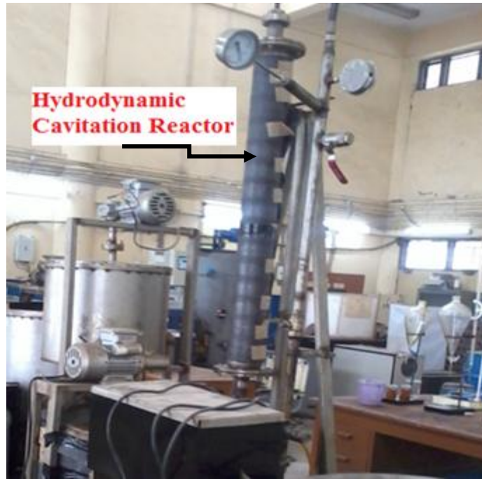
Figure 15. Hydrodynamic cavitation reactor experimental set-up
