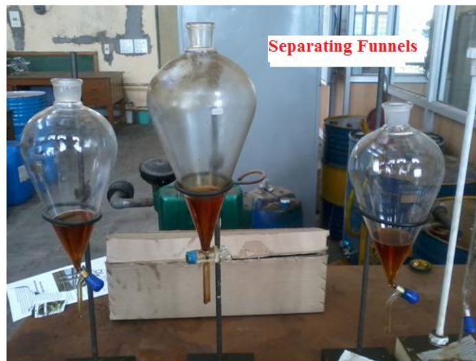
Figure 10. Glycerol separation process
