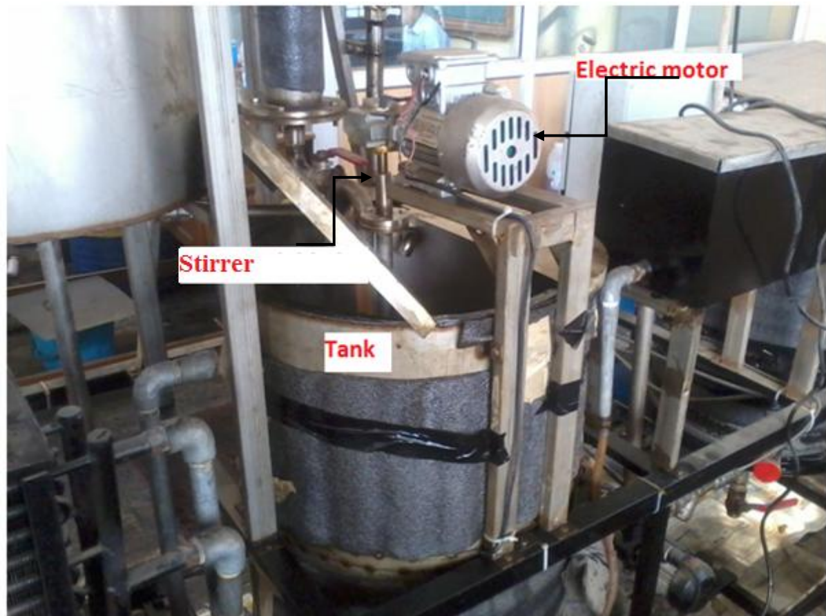
Figure 9. Experimental set-up of biodiesel reactor with mechanical stirrer
