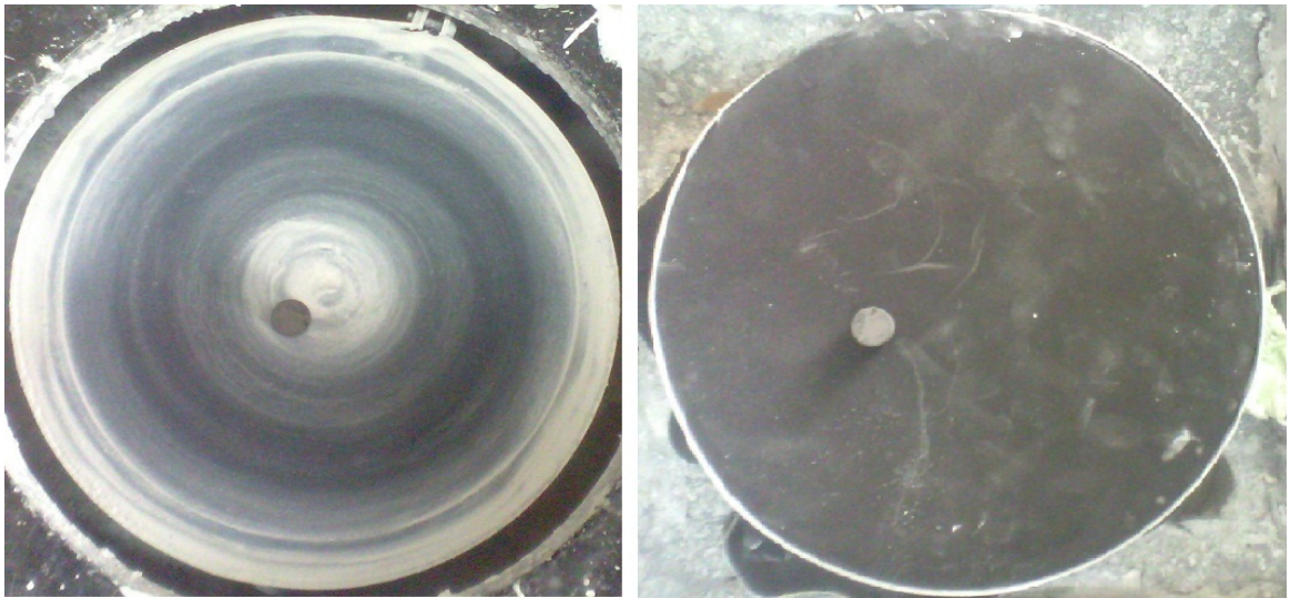
Fig 7.6 : Wet polishing and dry polishing of the sample specimen in metallurgy lab.
