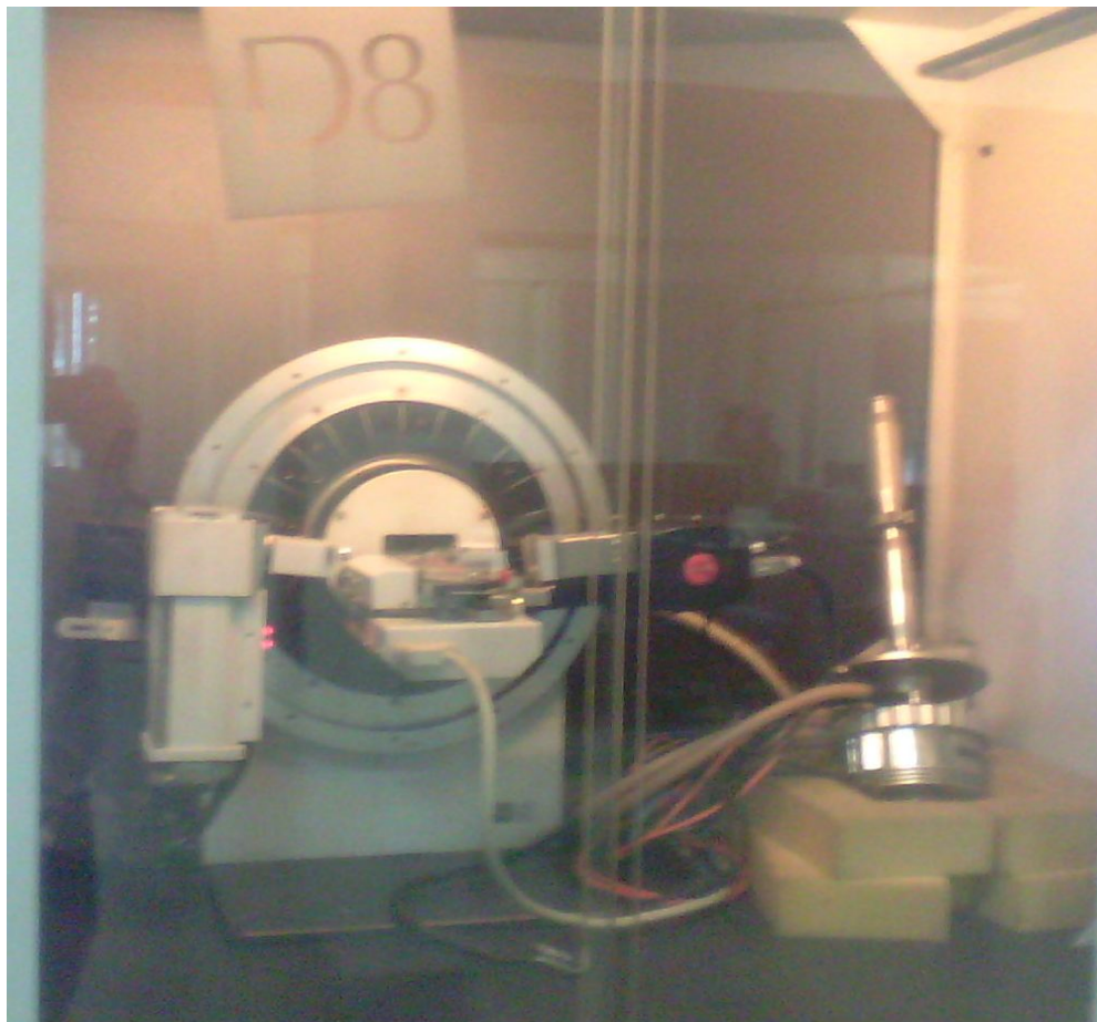
Fig 7.21 : XRD machine set up at IIT roorkee
