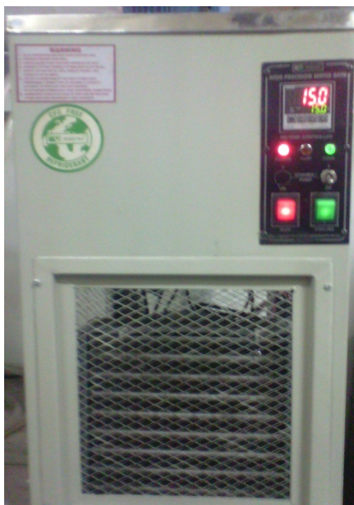
Fig 5.4: Chiller connected to the tube furnace to control the heating and cooling rate
