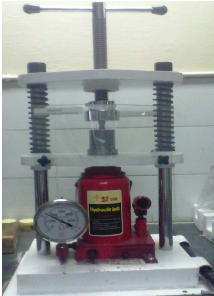
Fig 6.2 : Hydraulic jack set-up having 15 ton capacity
