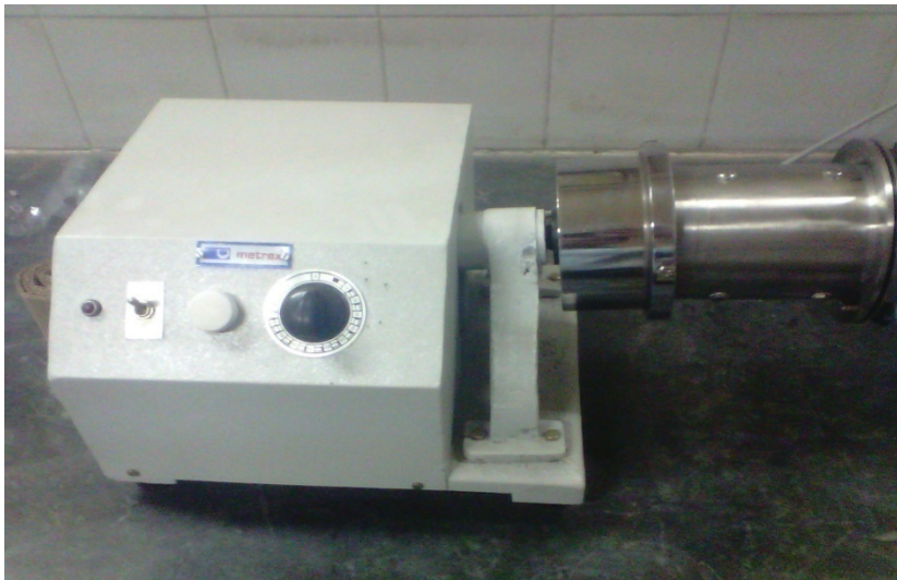
Fig 6.1 : Set-up of ball mill having automatic timer and variable speed facility.
