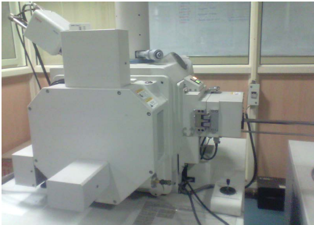
Fig 7.8 : Outlook view of the SEM machine connected with pump and computer
