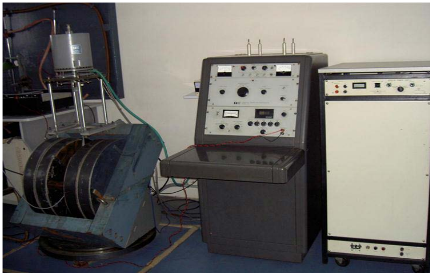
Fig 7.22 : VSM set-up at IIT Roorkee
