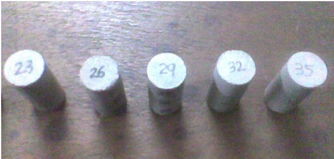
Fig 7.1 : Sintered specimen before fracture
