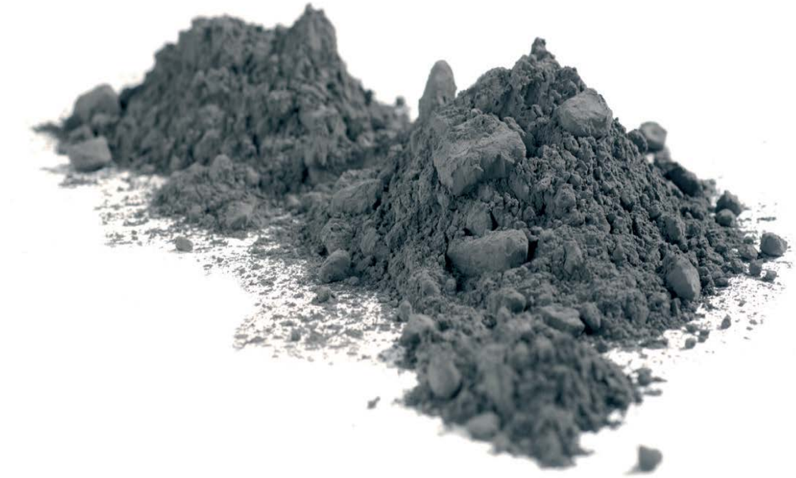
Fig 2.2: Carbonyl Iron Powder in the pure form
