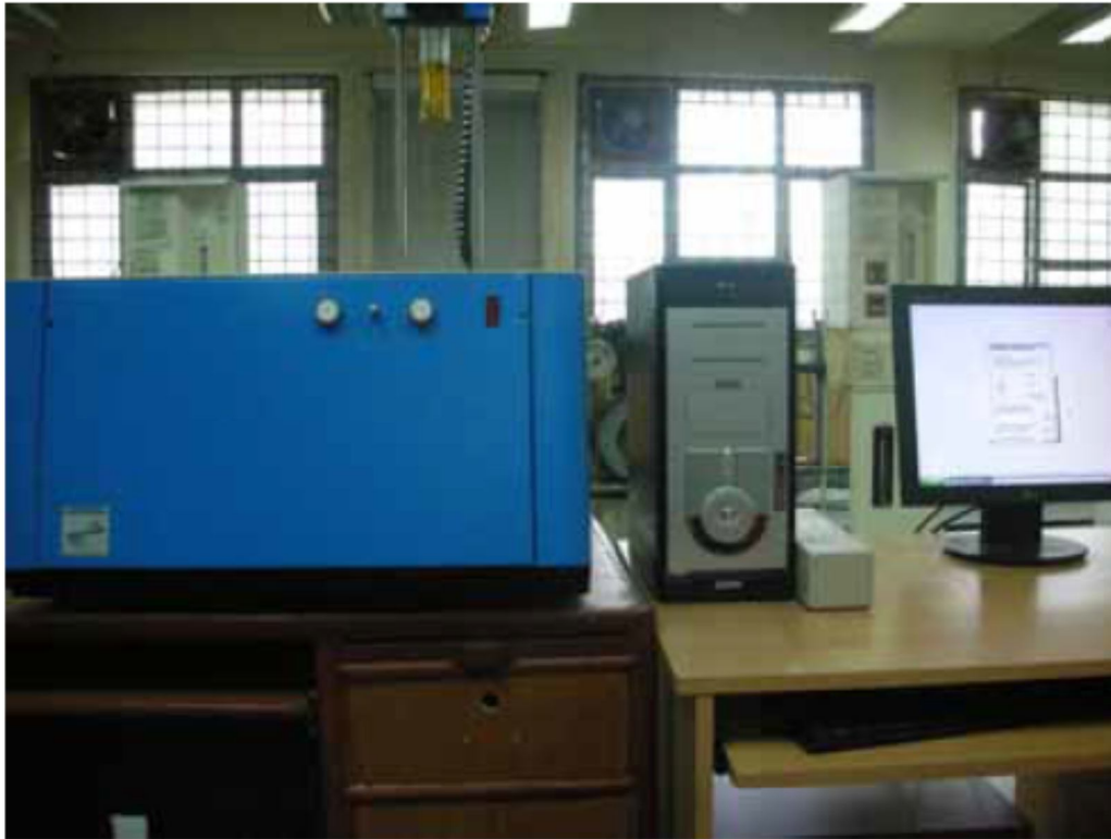
Plate 3.8 Cold Filter Plugging Point Apparatus
