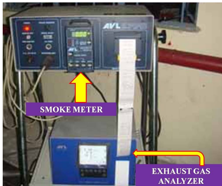
Plate 3.19 Exhaust gas analyzer and smoke meter
