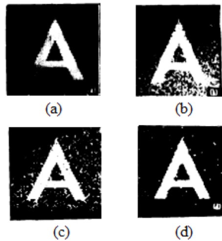
Figure 5.3: (a) Pure Image. (b) Image of 5.3(a) corrupted by N(0.100) noise. (c) Image after thresholding using 1D Otsu method. (d) Image after thresholding using 2D Otsu method
