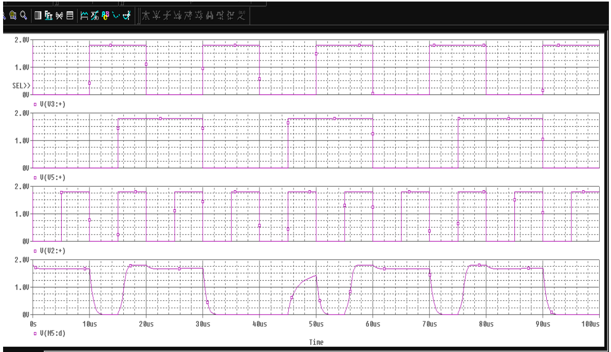
Fig 2.7 Output waveform of 2-input PDB AND domino logic.
