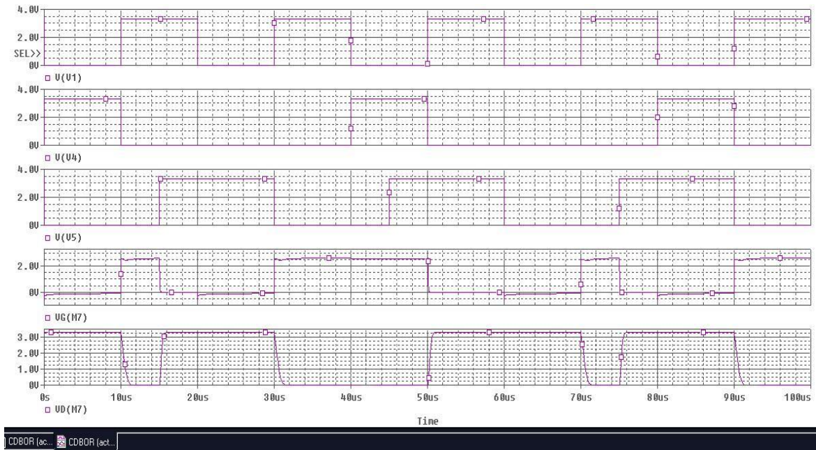
Fig 4.20 Output waveform of proposed 2-input OR/NOR domino logic.
