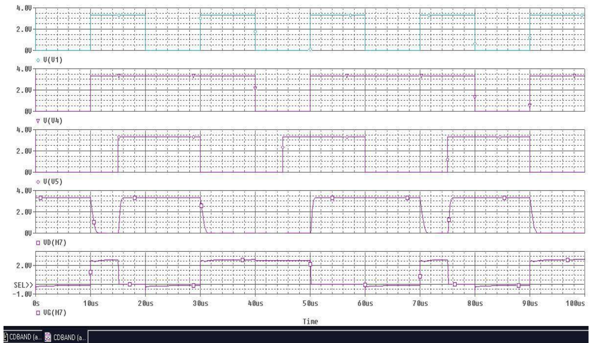
Fig 4.14 Output waveform of proposed AND/NAND domino logic.
