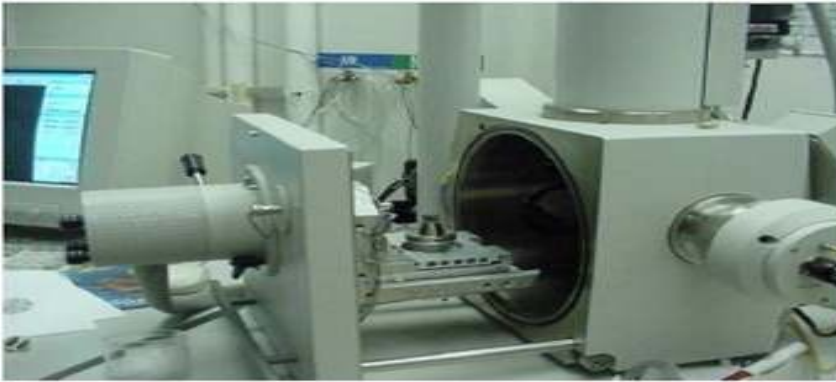
SEM opened sample chamber
