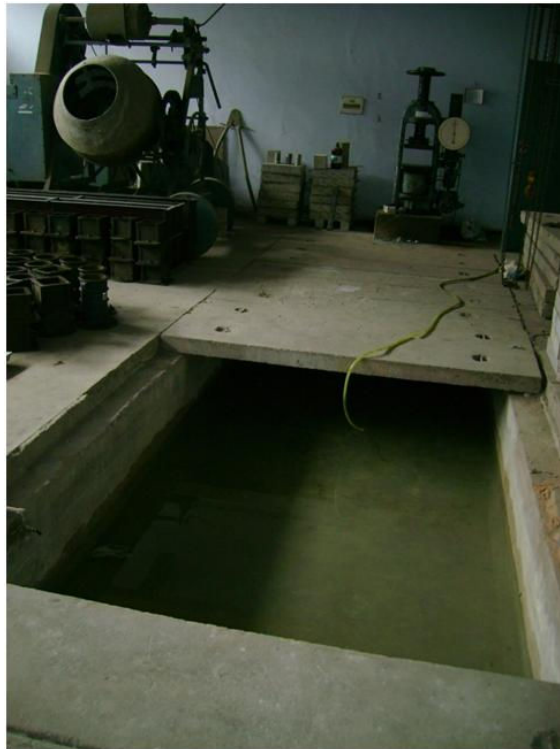
Fig. 36 Mechanical Mixer Capacity 0.5 cum and Curing Tank
