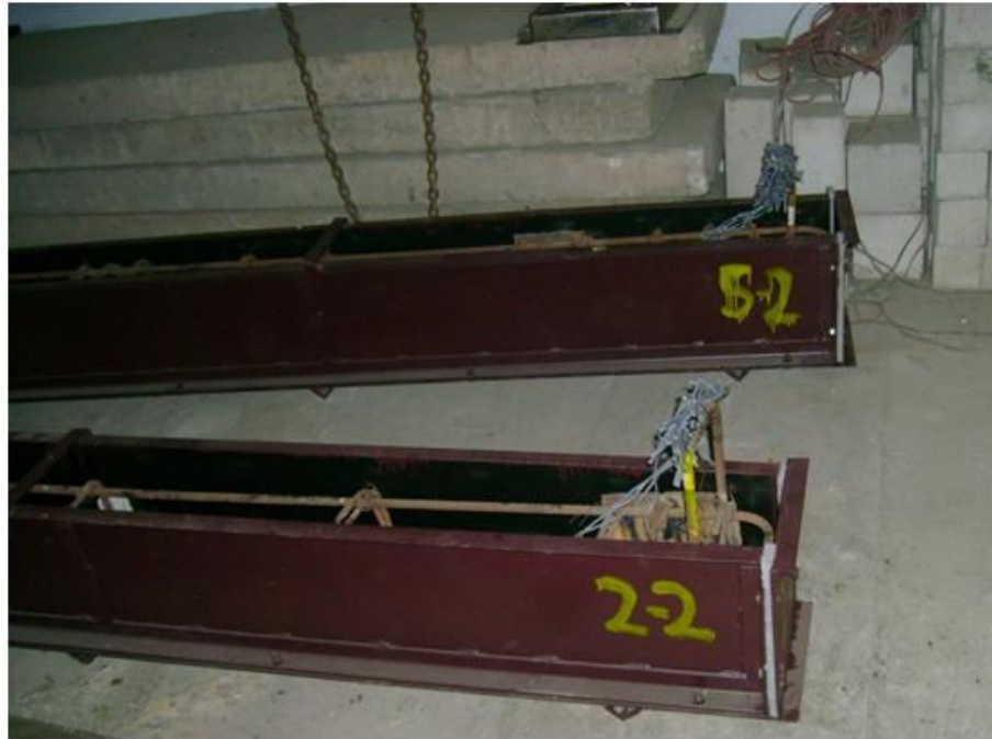
Fig. 37 Reinforcement Cage inside the Beam Mould
