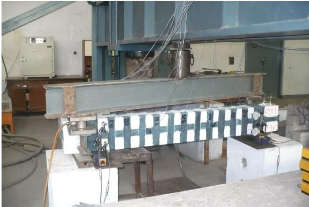
Fig. 64 Position of Dial Gauges to Measure the Twist Angle and Load Cells of PTT-1
