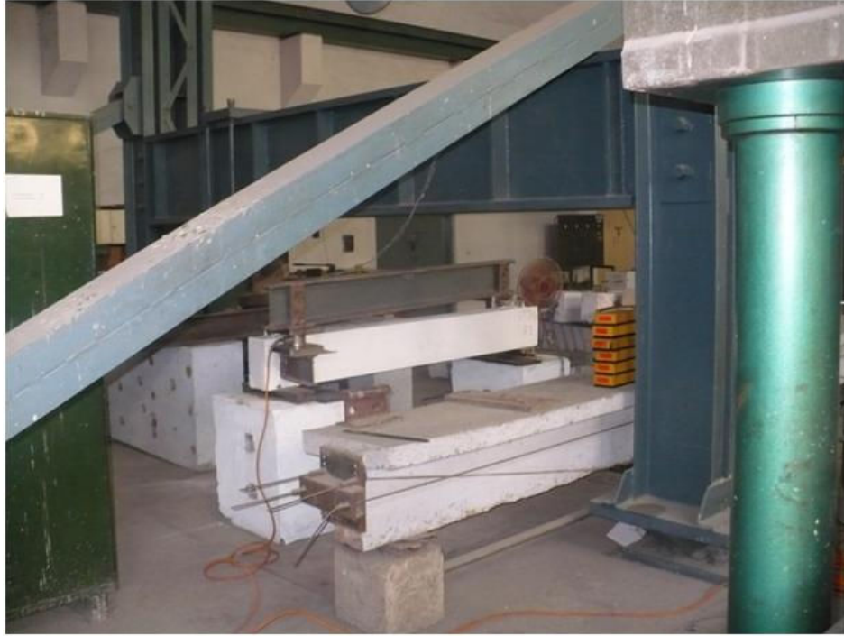
Fig. 60 Static 50 Tons Capacity Loading Frame
