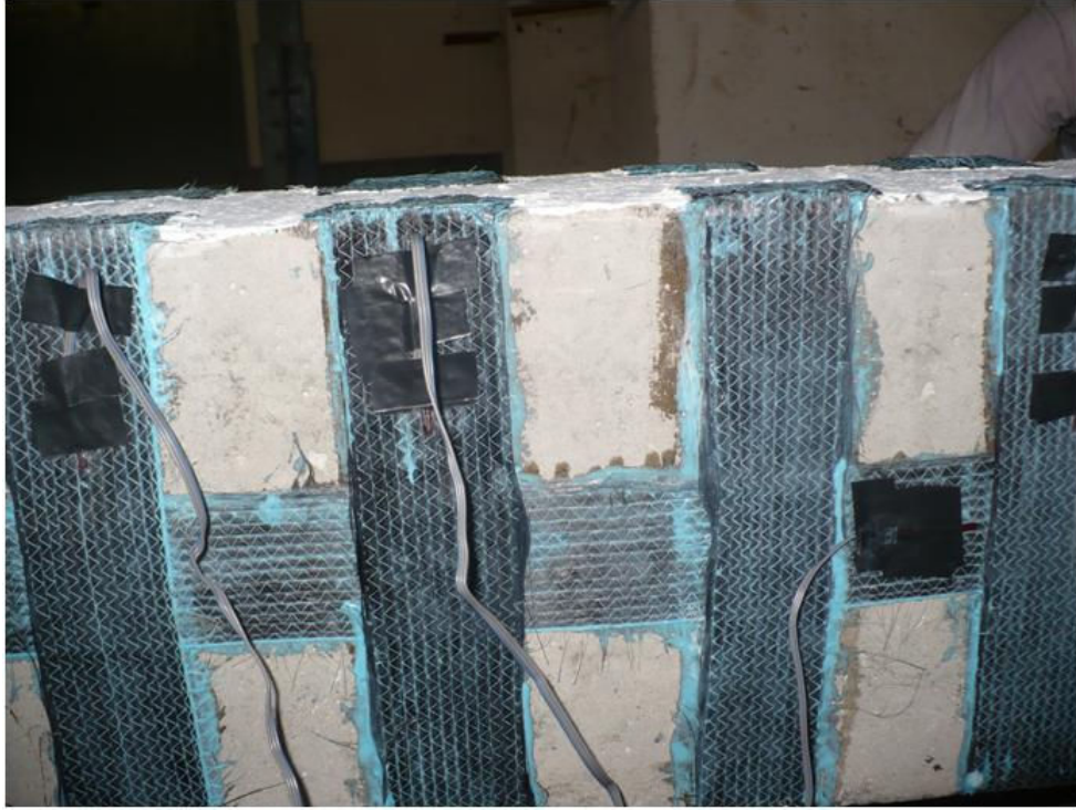
Fig. 58 Position of Electric Strain Gauges on Surface of CFRP Fabric
