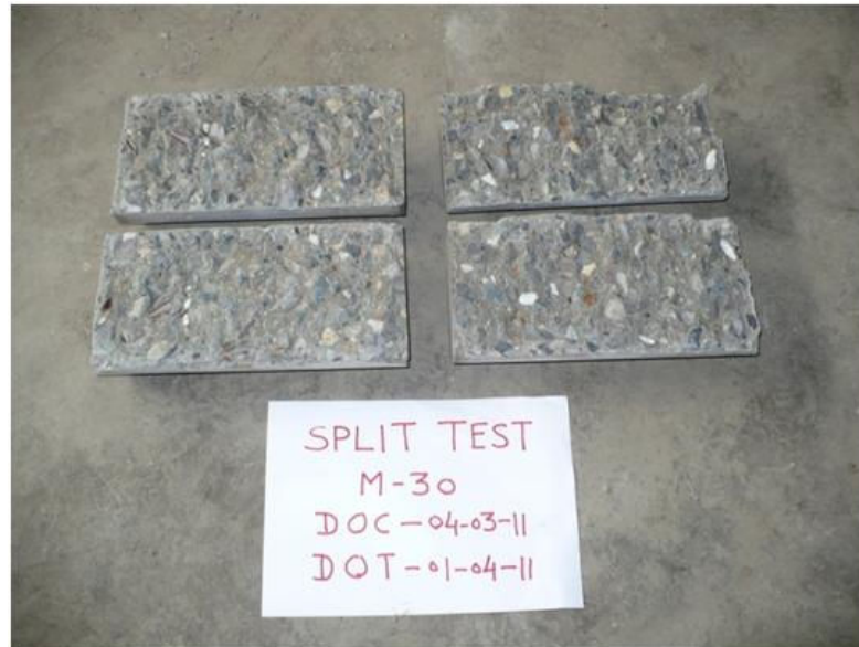
Fig. 47 Split Surface of Cylinder after Testing
