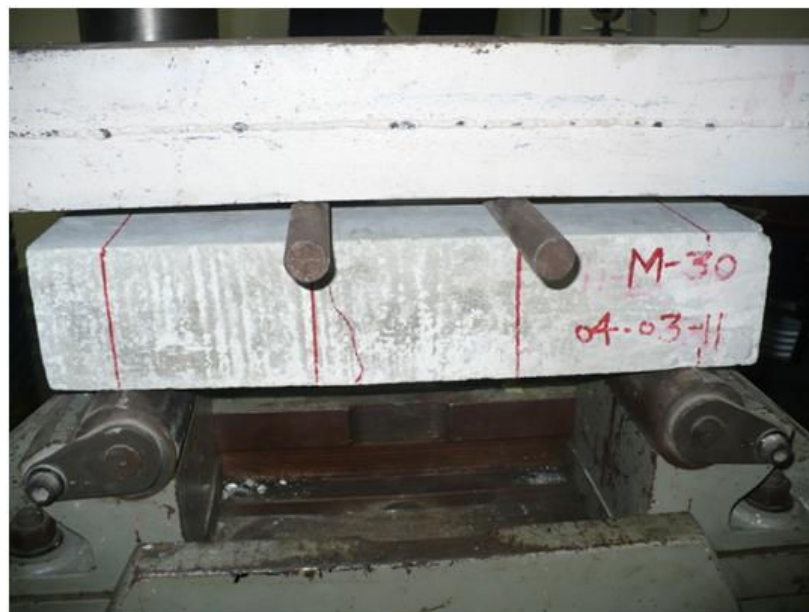
Fig. 50 Failure of Prism after Flexural Test
