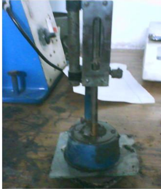
Fig. 9 Vicat's Apparatus showing Testing of Consistency of Cement
