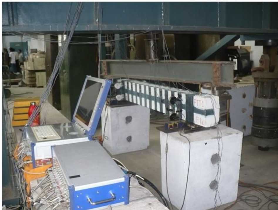
Fig. 79 Setup of the Test of the PTT-1 Beam
