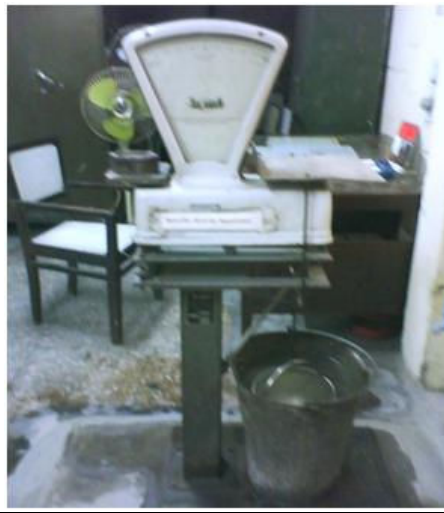
Fig. 15 Apparatus of Weighing of Aggregate in Water
