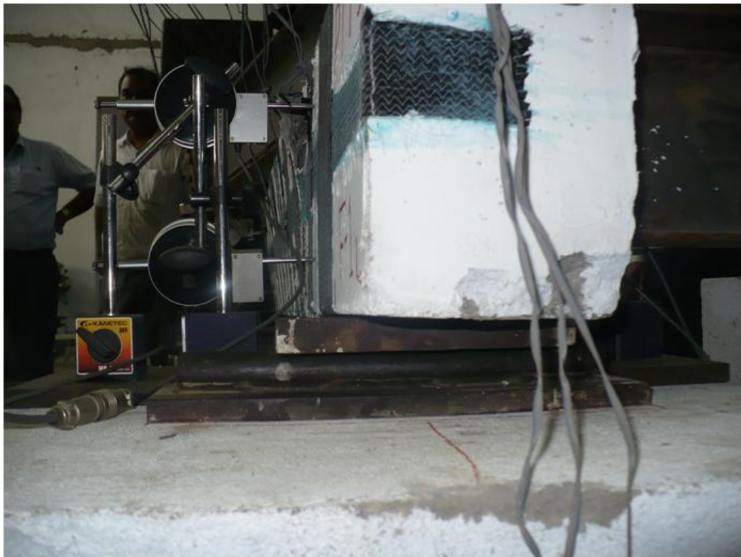
Fig. 84 Crushing Failure View from Roller End
