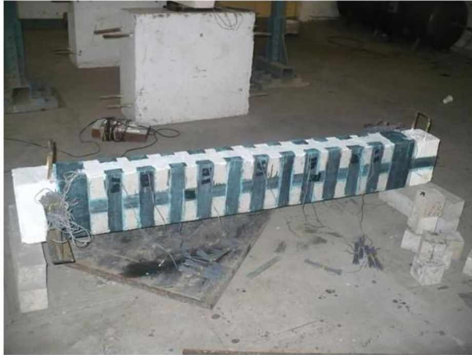
Fig. 55 Beam PTT-1 Strengthen with U-Shaped Wrapped of CFRP Fabric 50 mm Width 125 mm c/c with anchors and Longitudinal Strips
