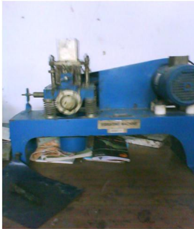
Fig. 12 Vibrating Machine for mixing of Cement Mortar Cubes
