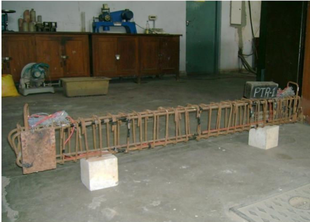
Fig. 30 Caging of RC Beam PTR – 1 Showing Reinforcement, Electric Strain Gauges and Steel Plates at Both Ends for Torsion Loading
