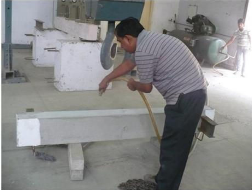
Fig. 51 Removing Loose Particles by Compressed Air
