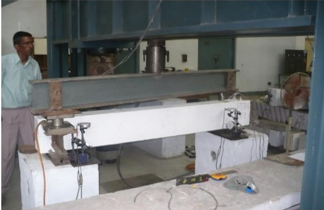
Fig. 63 Position of Dial Gauges to Measure the Twist Angle of and Load Cells of PTR-1
