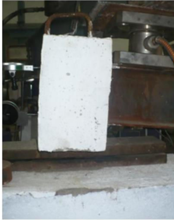
Fig. 68 Position of Twisted of Beam at Rocker End Cracks were formed (Torque was 10.68 kNm) at Face F-3
