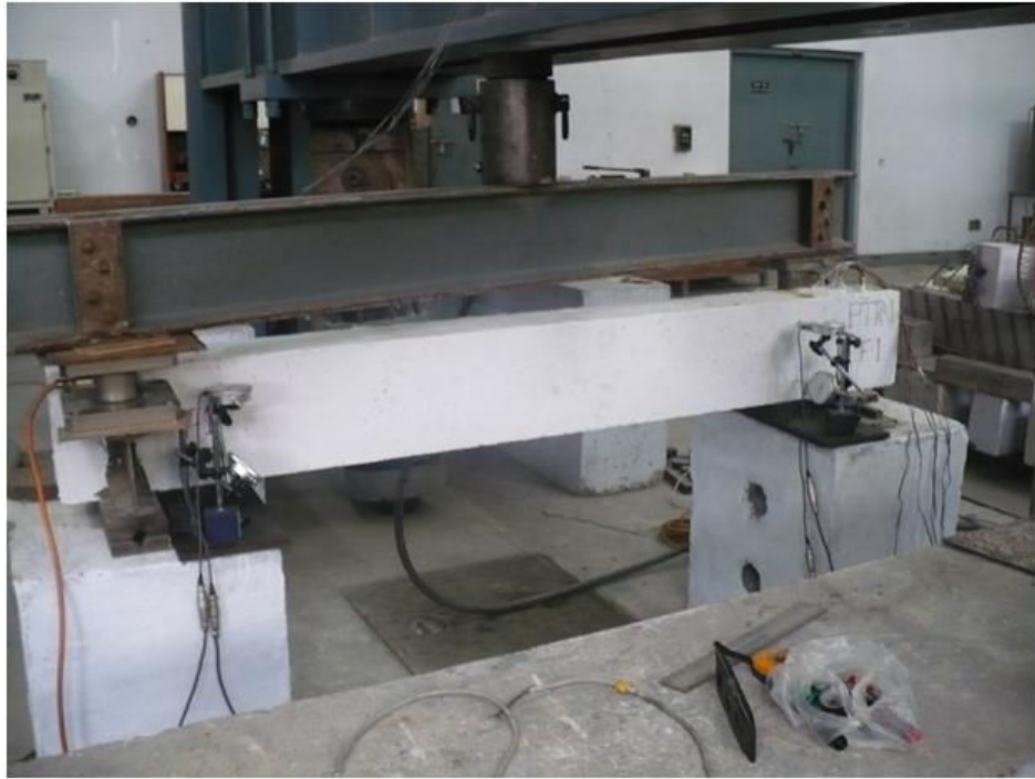
Fig. 61 Experimental Setup of Beam PTR-1
