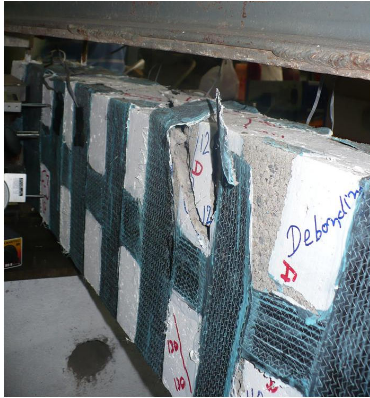
Fig. 85 Close View Crushing Failure of Concrete and Deboning of CFRP Fabric Strips
