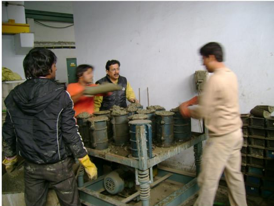
Fig. 42 Filling of Cylinders on the Table Vibrator
