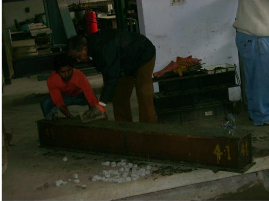
Fig. 41 Finishing of Top Surface of Beams
