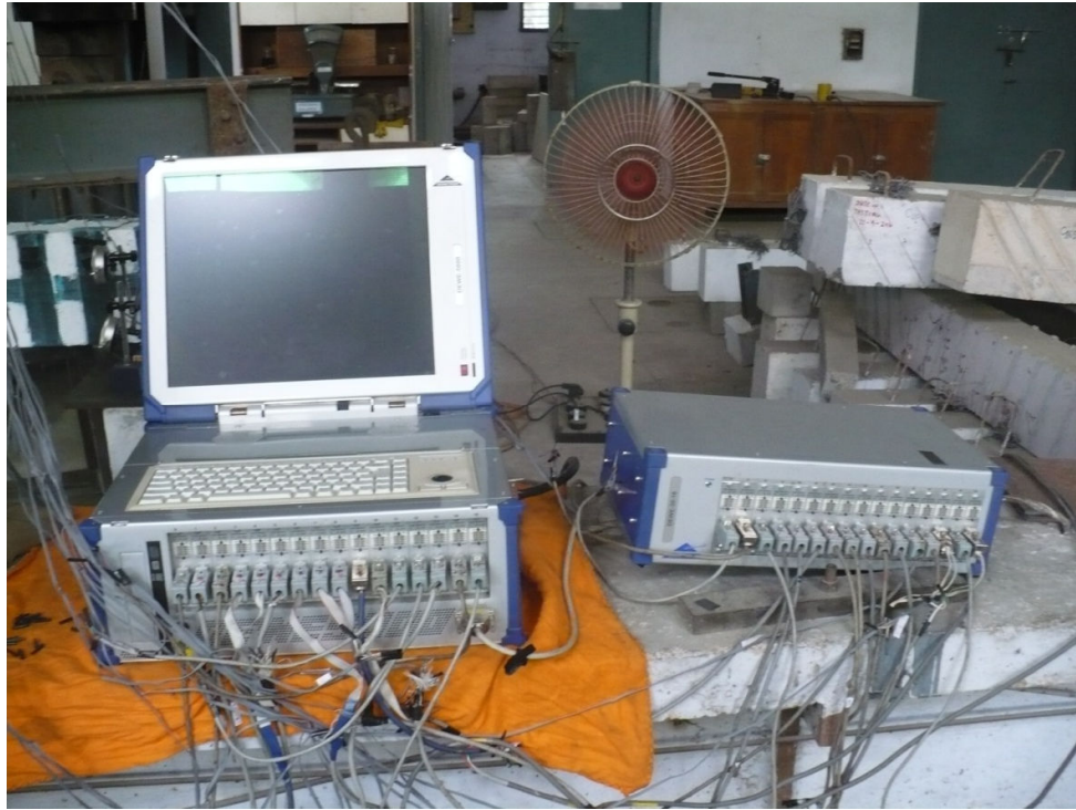
Fig. 65 Dynamic Data Logger “DEWETRON”-32 Channels
