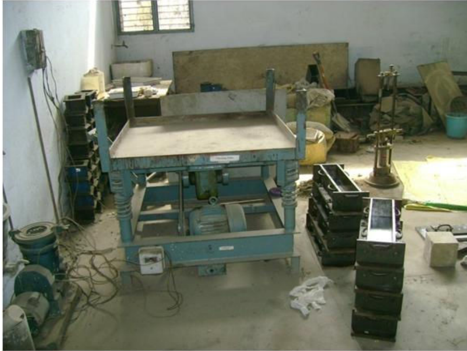
Fig. 35 Table Vibrator and Prism Moulds
