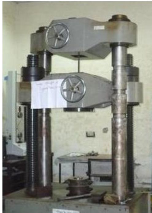
Fig. 22 Testing of Ultimate Tensile Strength of Steel Rebar
