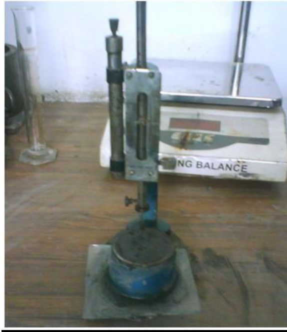
Fig. 10 Vicat's Apparatus showing Testing of Initial and Final Setting Time of Cement
