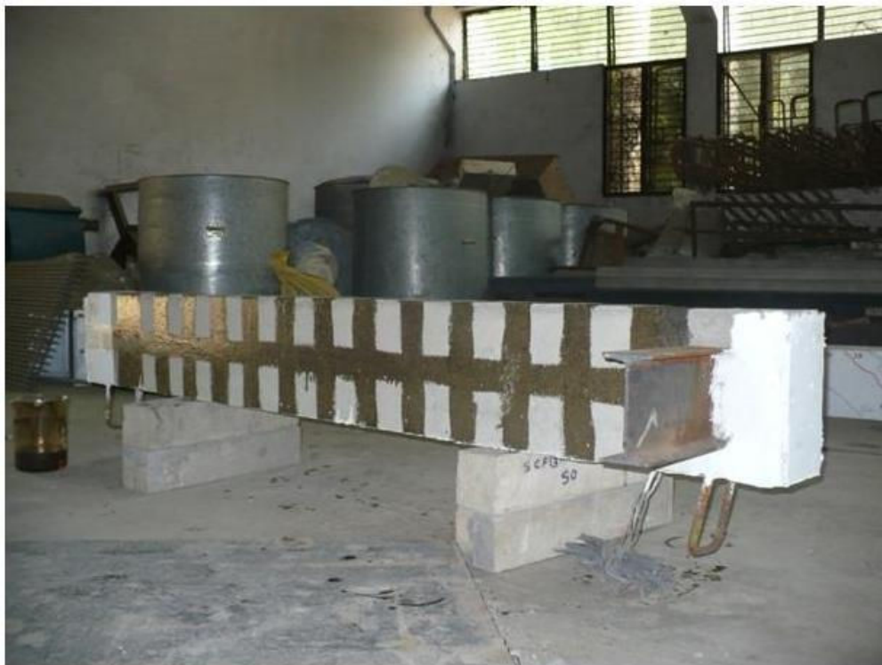
Fig. 52 Concrete Impregnated with R&M Resin Primer 11
