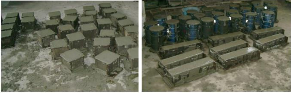
Fig. 43 View of Cubes, Cylinders and Prism after Concreting
