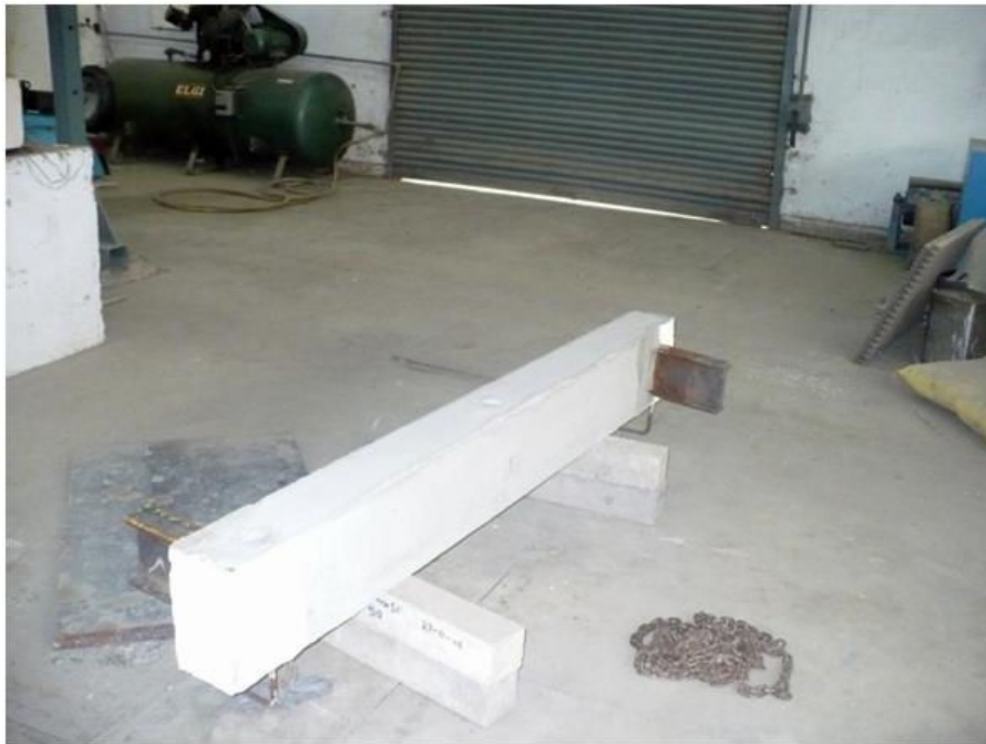
Fig. 59 Position of ISWB 150 Welded at End Plates for Torsional Loading
