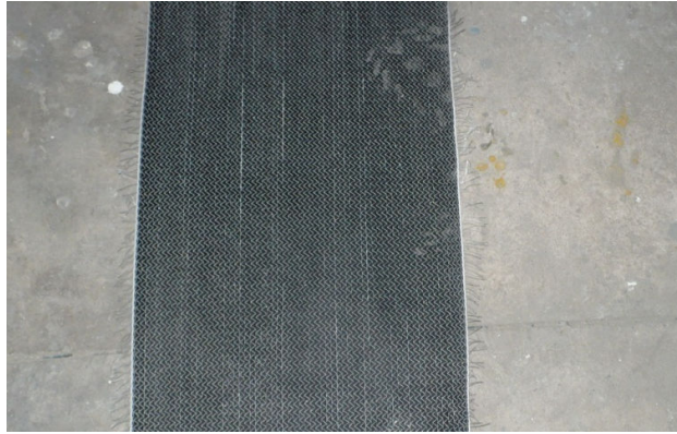
Fig. 23 CFRP-Fabric – 400 g/m 2 (Unidirectional)
