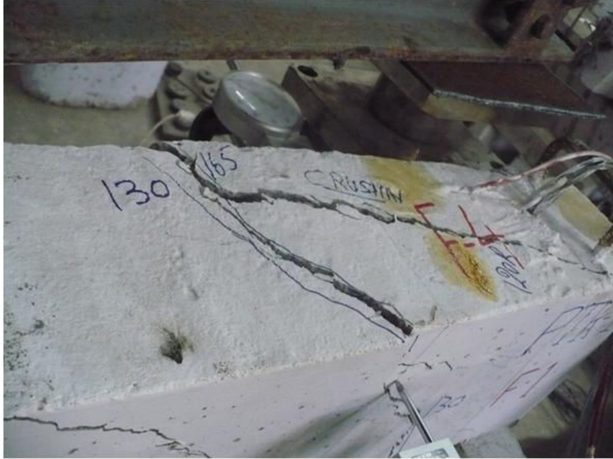
Fig. 70 Position of Cracks Total Load of 165 kN (Torque was 14.14 kNm) Face F-1 and F-4
