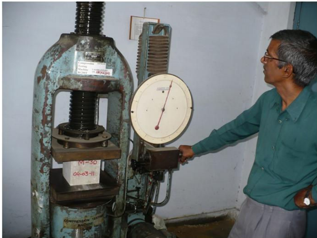
Fig. 44 Testing of Cubes for Compressive Strength
