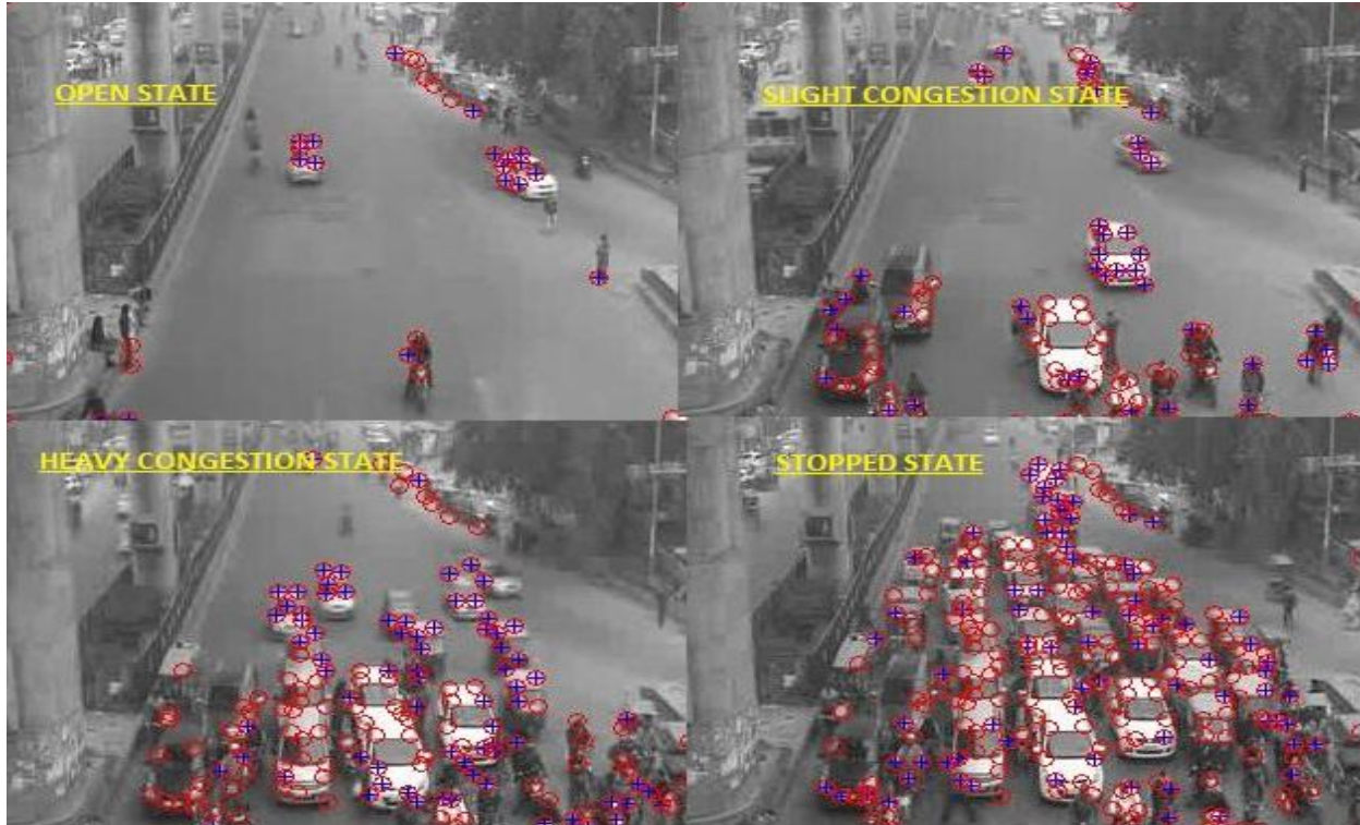
Figure 6.1: Each Frame illustrates a road traffic state, spatial and spatial temporal points in red and blues respectively.
