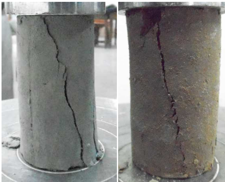
Fig. 3.24: Failure pattern of sample obtained in UCS test
