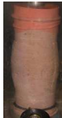
Fig. 3.30: Failure pattern of sample
