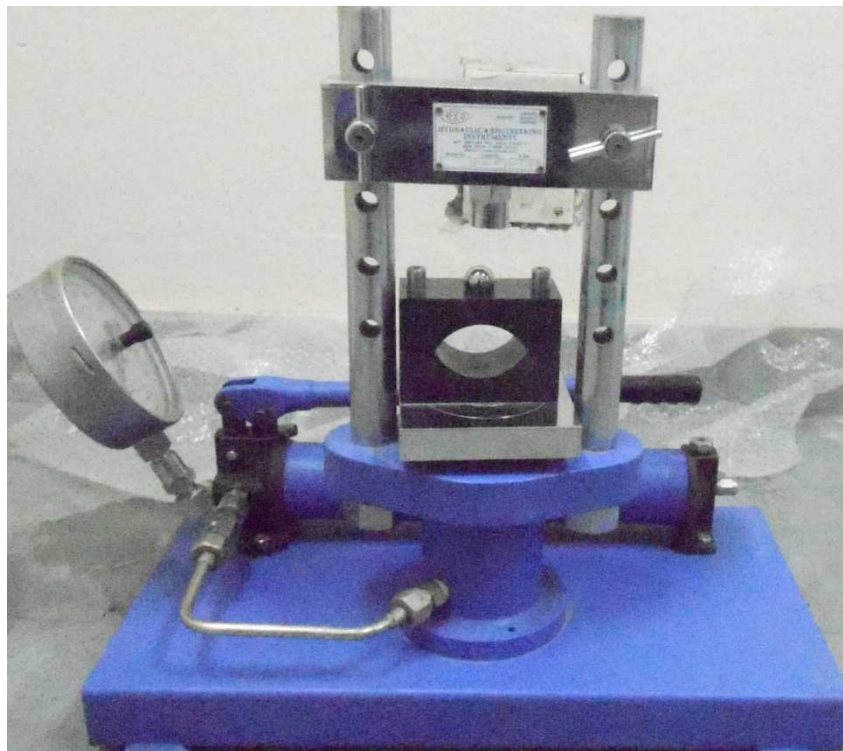
Fig. 3.37: Brazilian Test Apparatus
