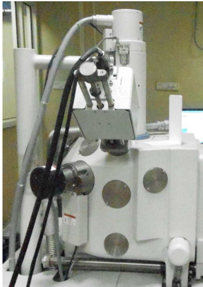
Fig. 3.6: Energy-Dispersive Spectrometer in SEM
