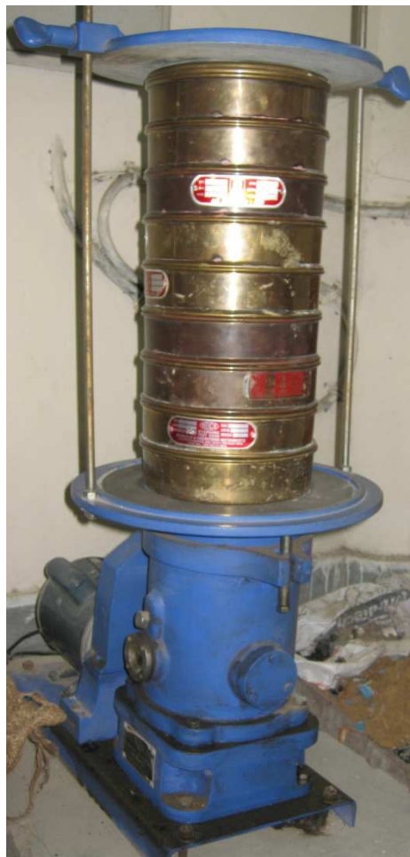
Fig. 3.11: Sieves with Mechanical shaker used for sieve analysis
