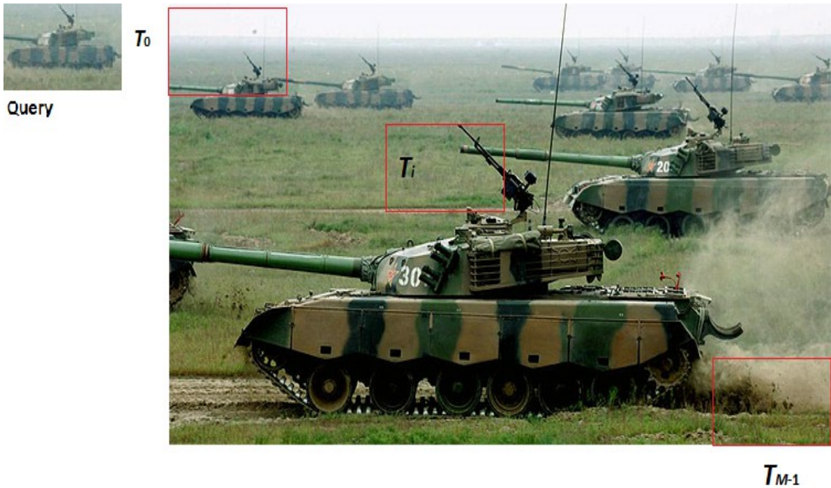
Figure 1.1: Given a query image Q , we want to detect/localize objects of interest in a target image T . T is divided into a set of overlapping patches.
