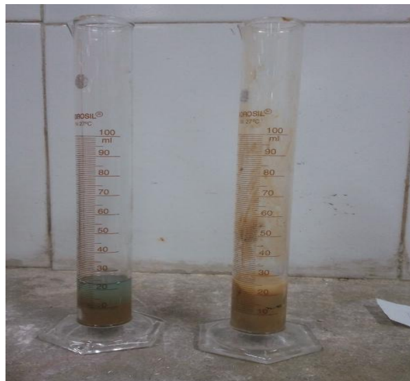
Image 3.7: Free swell Ratio test
