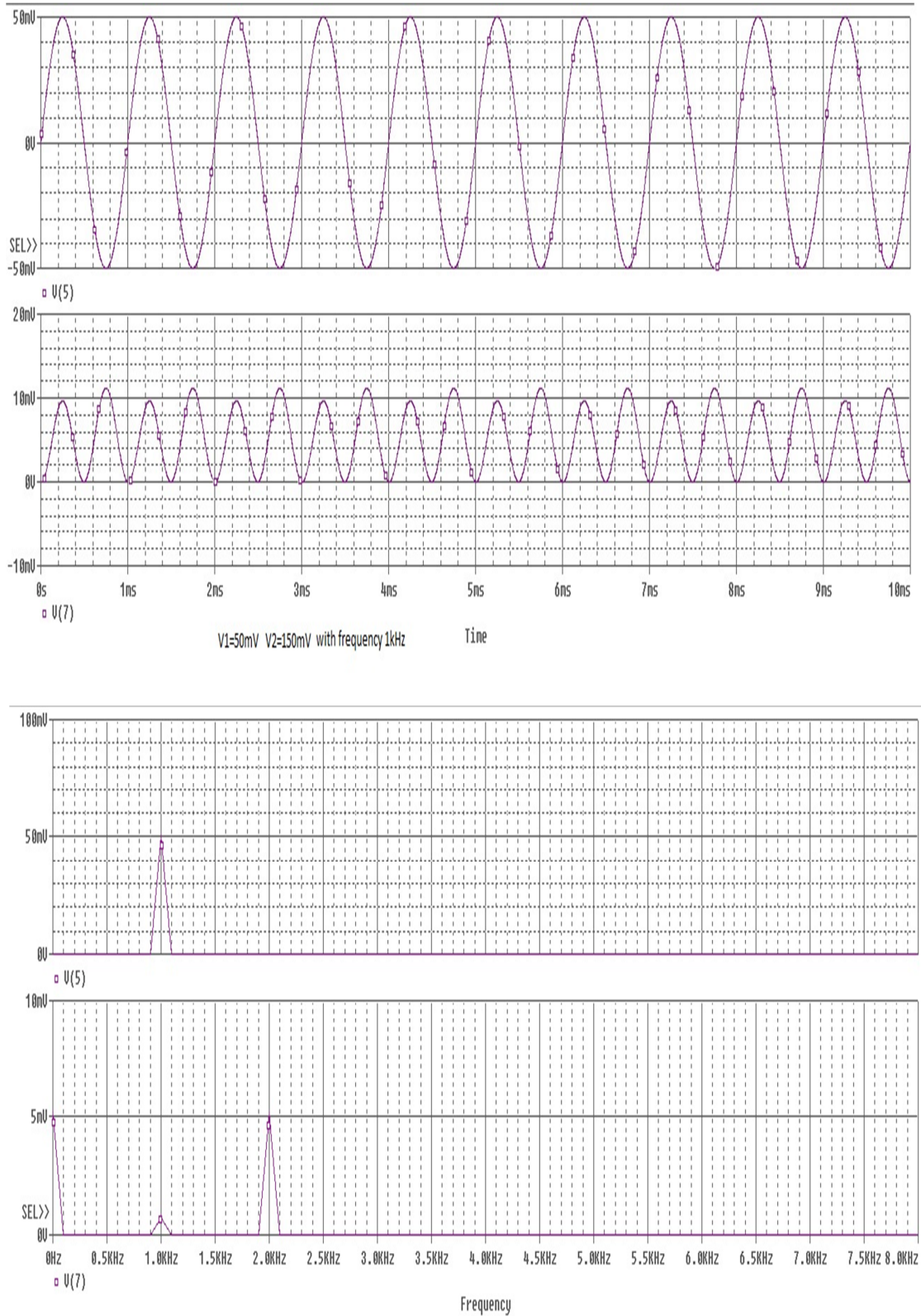
Fig. 2.17 Input and Output of multiplier circuit at f_1=f_2=1 KHz
