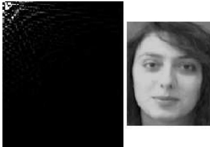
Figure 2.6 DCT of a Face image
