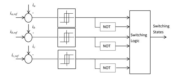
Fig. Structure of Hysteresis Current Controller
