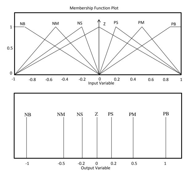
Fig. 3.6 Input and Output membership function representation
