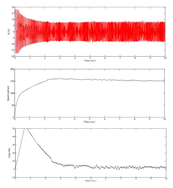
Fig. 4.7 Experimental Performance of IVCIM using PI controller with Hysteresis Band=5 in current controller
