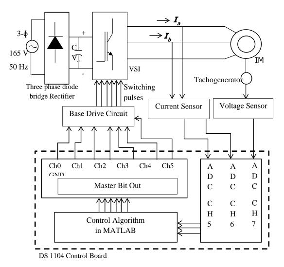
Fig. 3.1 Block Diagram of the complete hardware scheme
