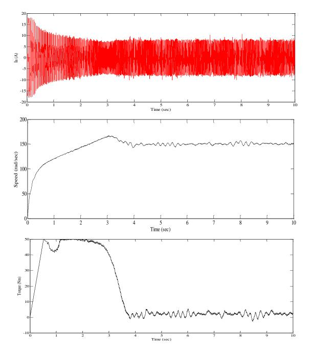
Fig. 4.11 Experimental Performance of IVCIM using FLC with Hysteresis Band=5 in current controller
