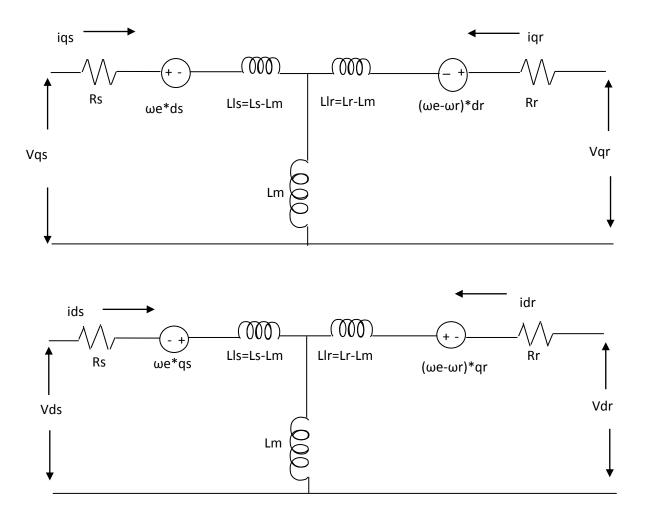
Fig. 2.2 Equivalent circuit of Induction motor in a synchronously rotating reference frame, a) quadrature-axis circuit b) direct-axis circuit
