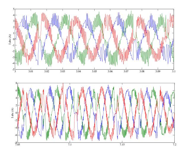
Fig. 4.9 Steady state value of line currents  $(i_a, i_b, i_c)$  at (a) no load (b) load
