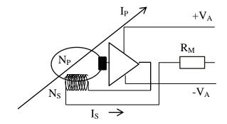
Fig. Principal Diagram of ABB Current Sensor
