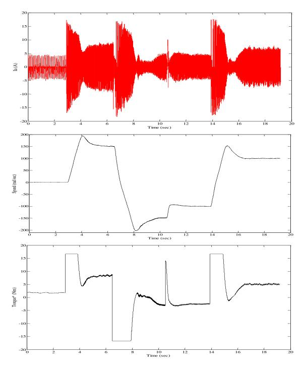
Fig. 4.6 Experimental Performance of IVCIM using PI controller in forward, reverse and braking mode
