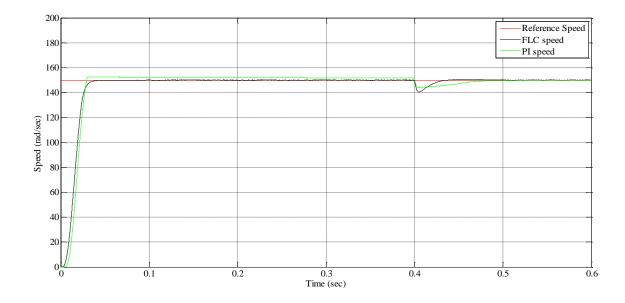
Fig. 4.12 Comparison of Speed deviation in PI & Fuzzy Logic Controllers
