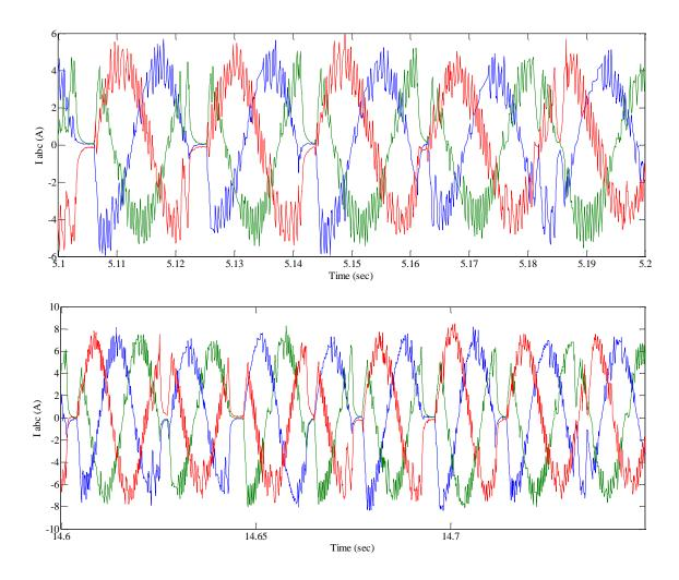
Fig. 4.5 Steady state value of line currents (i<sub>a</sub>, i<sub>b</sub>, i<sub>c</sub>) at (a) no load (b) load
