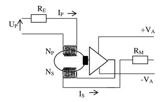
Fig. Principal diagram of EM010 Sensor
