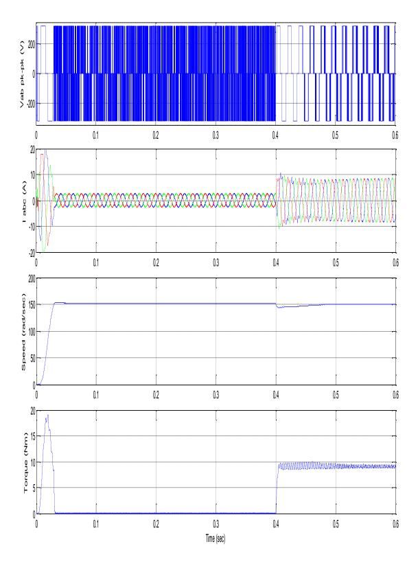
Fig. 4.2 Performance analysis of IVCIM using PI controller for (a) no load (b) load applied at t=0.4 sec
