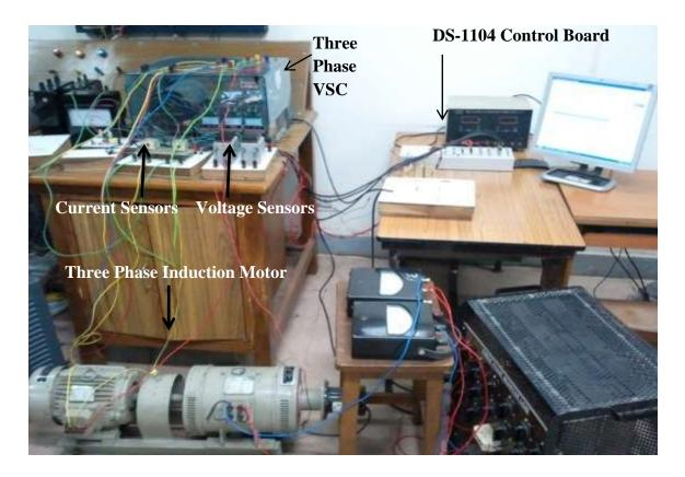
Fig. 3.3 Hardware setup for indirect vector control drive for 3 Hp, 230 V, 1440 rpm IM
