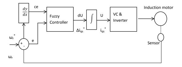
Fig. 3.5 Functional block diagram of Fuzzy Logic Controller
