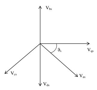
Fig. 2.3 abc-dq axes transformation in synchronously rotating frame of reference
