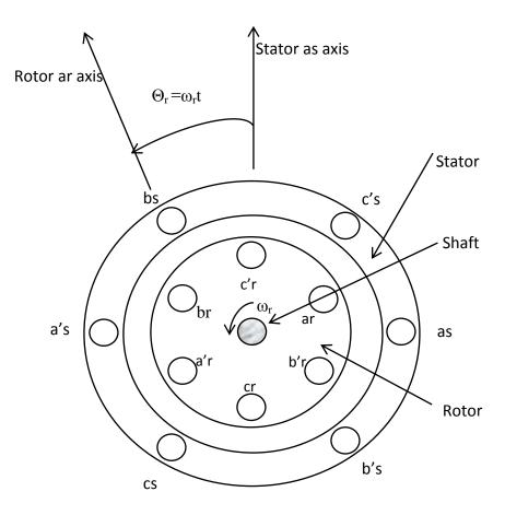
Fig. 2.1 Representation of a three phase induction motor
