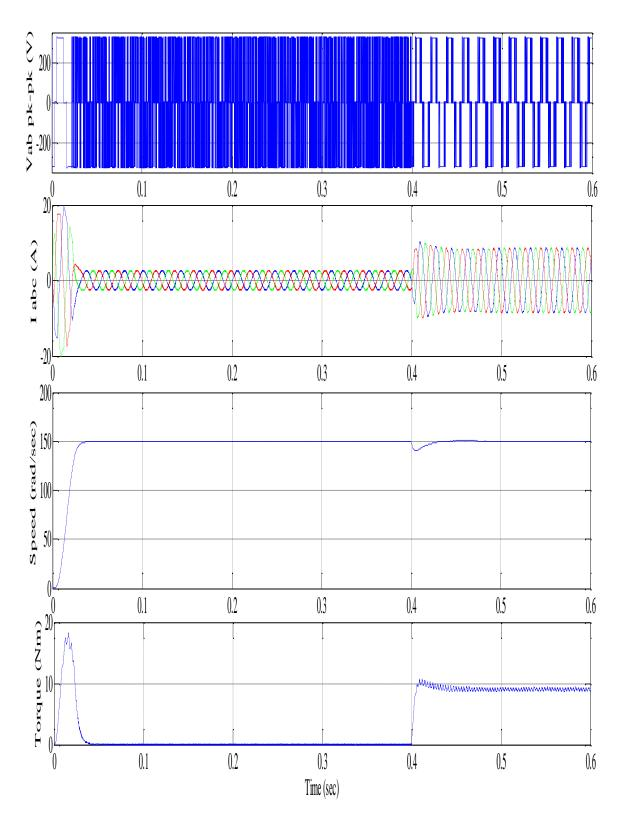
Fig. 4.3 Performance analysis of IVCIM using FLC for (a) no load (b) load applied at t=0.4 sec
