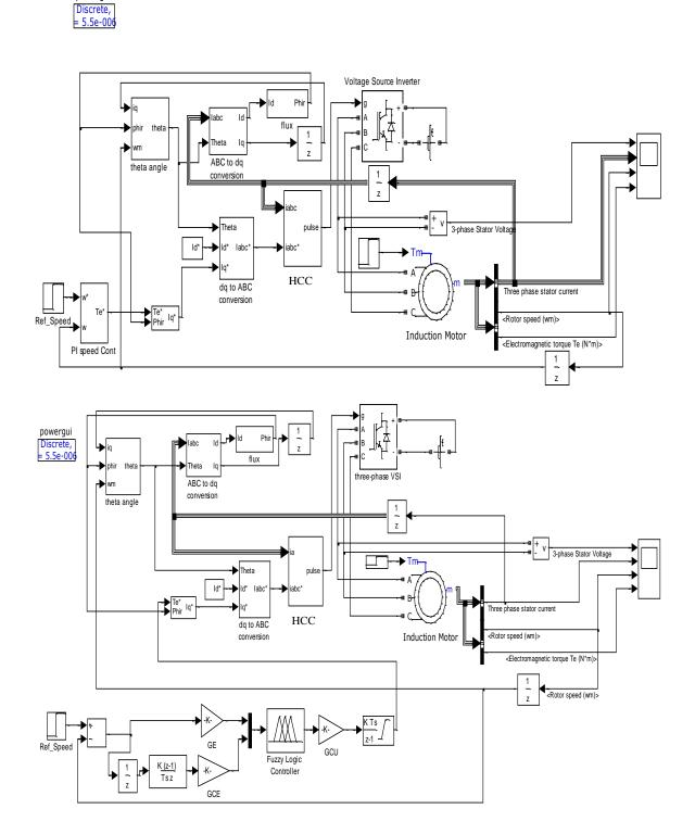
Fig. 4.1 Simulink Model of IVCIM with (a) PI Controller (b) Fuzzy Logic Controller
