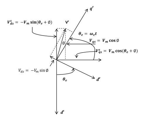
Fig. 2.5 Stationary frame to synchronously rotating frame transformation
