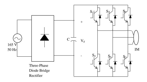
Fig. 3.2 Voltage Source Converter (IGBT based)
