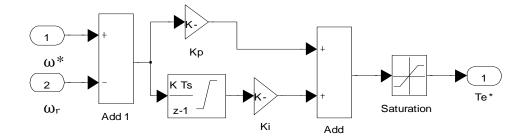
Fig.3.4 Proportional Integral Controller block diagram
