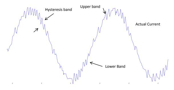
Fig. An actual current waveform obtained from Hysteresis Current Control
