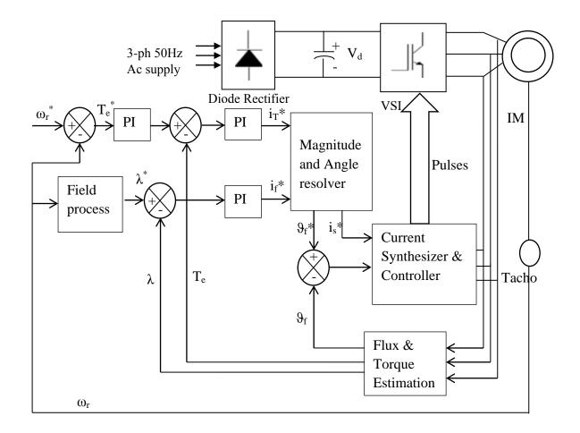
Fig. 2.6 Block diagram representing direct vector control scheme
