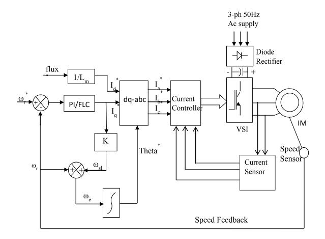
Fig. 2.7 Block Diagram representing Indirect Vector Control Scheme
