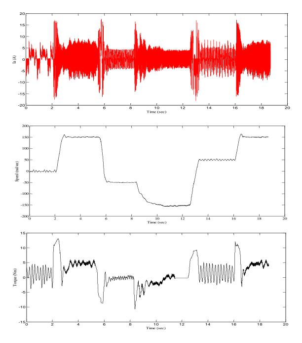
Fig. 4.10 Experimental Performance of IVCIM using FLC in forward, reverse and braking mode
