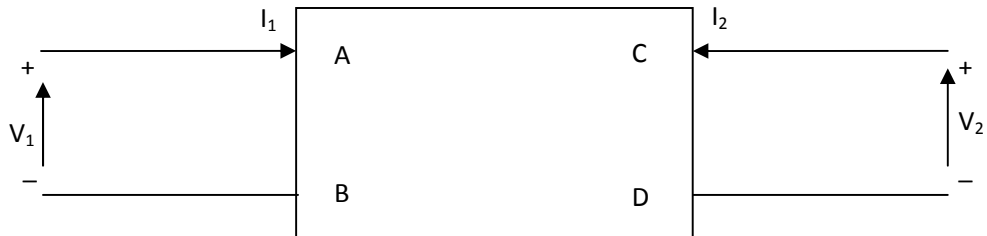
Figure 2.6 ABCD Parameters of Two port Network
