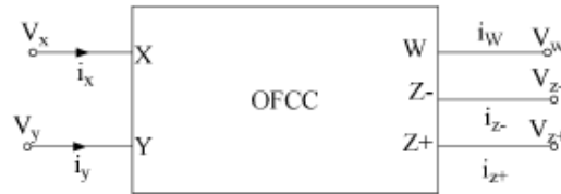
Fig 2.5 Block diagram representation of OFCC
