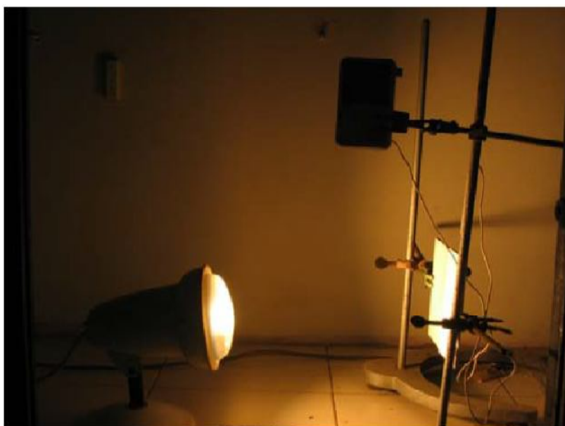
Experimental setup for measuring the infrared reflectivity of pigments
